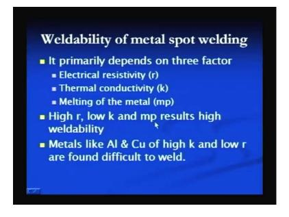
The weldability of a given material by the spot welding to a great extent is determined by the electrical resistivity, thermal conductivity, and the melting point. These are the 3 main parameters that affect the weldability of the metal by spot welding and that is why weldability of the metal by spot welding is calculated using equation which is based on the electrical resistivity r, the thermal conductivity k and melting point p.
