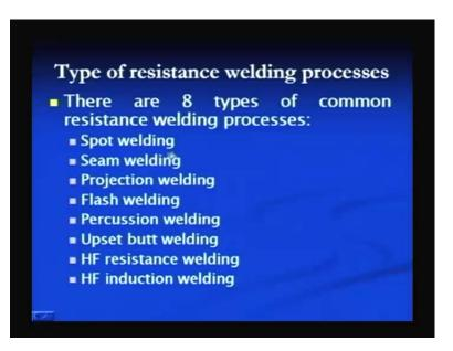
There are various types of the resistance welding processes which are used in different industrial applications, but the eight are the common one, and out of these eights, here the first 3 types of resistance welding processes are the most common and others are used in very specific areas.
