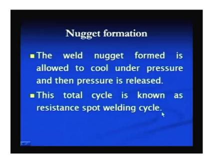
And when the nugget is formed, weld nugget is formed, it is allowed to cool under pressure and then pressure is released gracefully. These are the four steps in producing the joint by spot welding, and the entire, all these four steps are termed as resistance spot welding cycle.
