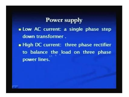
And power supply for the resistance spot welding process can be of low AC value or the high DC value. Low AC current is supplied using a single phase step down transformer and the high DC current supplied using 3 phase rectifier to balance the load of 3 phase supply.
