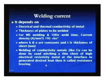
Out of the factors which significantly affect the selection of the welding current are electrical and thermal conductivity of the metal. If the electrical and thermal conductivity of a given metal is high, then we will require higher welding current because whatever heat is generated at the interface, that will be dissipated easily because of high thermal conductivity. And due to the high electrical conductivity, the heat generated at the interface will be less.
