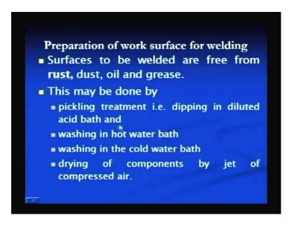
For producing a successful joint, sound joint, the surface must be free from the impurities and the dust and dirt. If the rust is present, or dust and oil and grease is present, these must be removed by using the suitable techniques. If the rust is present at the surface, we should follow this procedure like, pickling treatment is done first by dipping in dilute acid bath and then washing in hot water bath, washing in cold water bath and followed by drying using the compressed air jet.
