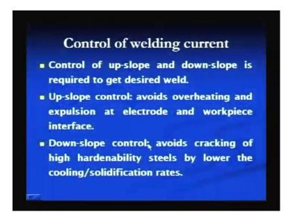
Welding current is to be controlled properly to avoid the defects and to form the sound weld joint like the rate of increase in current and the rate of decrease in current, that is termed as up slope and down slope should be controlled to get the desired weld. Up slope should be controlled to avoid the overheating between the electrode and the work piece surface, and also to avoid the expulsion between the interface of the work piece and interface between the electrode and the work piece.
