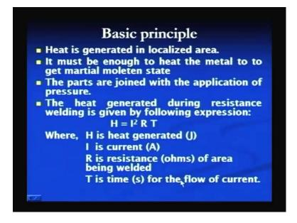
The basic principle of the resistance welding process lies in generation of heat by the electrical resistance heating in very localized manner. Heat is mainly generated in the
