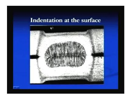
We can see here, the depression formed or the indentation formed at the surface of the work piece due to the heavy pressure transferred from the electrode to the work piece surface. This indentation can reduce the steam value of the product or can damage to the surface of the work piece.
