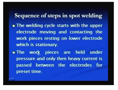
So, weld cycle starts with the upper electrode moving and contacting the work piece, resting on the lower electrode which is stationary and work pieces are held under pressure and then flow of current is started for preset time.
