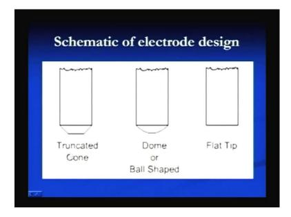
We can see 3 different shapes of the electrodes which are used in spot welding truncated cone, dome shaped or flat tipped electrodes.
