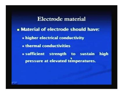
Materials of the electrode should have certain characteristics; means these electrodes are made of certain materials which can offer very good thermal and electrical conductivity, and having ability to withstand under the pressure because pressure is to be transferred through the electrode onto the work piece. So, these electrode materials must be strong enough to sustain high pressure at elevated temperature.
