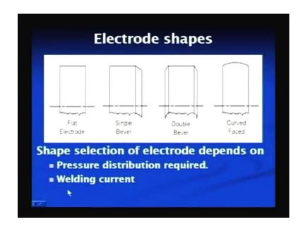
These are the different shapes of the rollers which are used in seam welding and these are the points which are to be considered, the kind of pressure distribution required, and the welding current which is to be used based on that we select a particular geometry of the roller to be used for.
