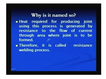
Why it is called so? Because heat required for producing the joint by using this process is generated by the flow of a, generated by the resistance to the flow of current through the contact area where joint is to be formed. And therefore, this processes is called resistance welding process.
