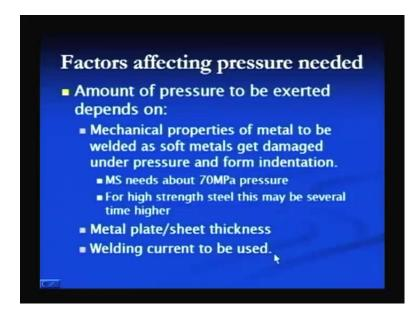
The amount of pressure which is to be exerted depends upon the mechanical properties of the material to be welded; stronger the material greater will the pressure required for producing this sound joint. Mechanical properties of the metal to be welded affect the pressure which is to be used for producing the sound joint. Soft materials may get damaged under pressure and form the indentation.
