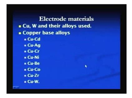
These are the common materials which are used for making the spot welding electrodes. These are basically Copper or Tungsten base alloys because both these materials show good thermal conductivity and electrical conductivity, but addition of the alloying elements in turn reduces the electrical conductivity, but these additions are frequently used to increase the strength of the Copper base alloys particularly.
