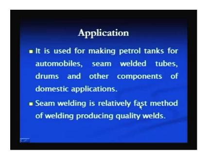
The application of the seam welding includes like a making the petrol tanks for automobiles, seam welded tubes, drums and other components for domestic applications and seam welding is relatively fast method for producing the high quality welds.
