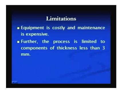
So, here, now we can see that some of the limitations also there with these equipments. Like equipments are costly and maintenance is also expensive. For these processes are limited to the thin sheets, very thick sheets cannot be processed by the resistance welding processes, particularly seam welding and a spot welding.
