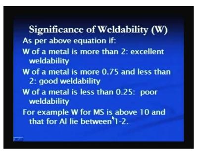
The weldability W can be calculated using above equation, can be interpreted in terms of the how easily we can weld a given material by this spot welding process. If the W of material comes more than 2, it shows the excellent weldability and if the W of material is in between 0.75 and 2, then it is considered a good weldability. If the W value becomes less than 0.25, then it is considered of poor weldability.
