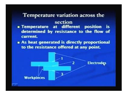
The temperature at different position is found different and it is mainly determined by the resistance to the flow of current in the different zones. As heat is generated, heat generated is directly proportional to the resistance offered by any point in the section which is being welded, and accordingly the temperature of that particular zone is determined; higher the resistance for a given flow of current greater is the temperature which is noticed.
