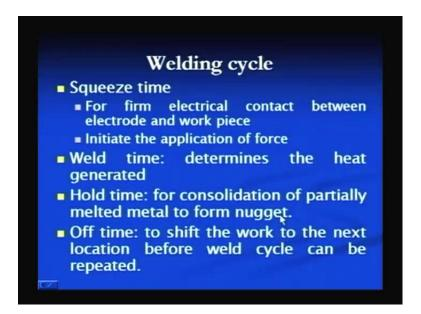
If we have to see, then it includes the squeezing times; the time for which the initial pressure is applied and during which pressure increases from zero value to the maximum squeezing pressure. This is applied for firm electrical contact between the electrode and
