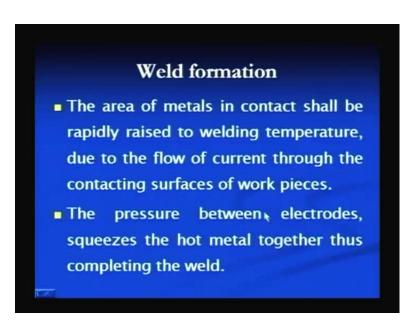
And when flow of current starts, it generates heat at the interface and the maximum heat is generated at the interface and which leads to the partial melting of the work pieces of surfaces at the interface. And under pressure, the molten metal is squeezed and consolidated to form nugget.
