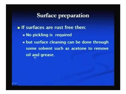
And if the surface is free from the rust, then pickling is not required. But only surface cleaning is done using the acetone to remove the oil and grease from the surface.
