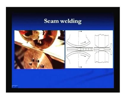
Here, we can see more clearly. This is a upper roller, lower roller, and these are the two plates which are to be welded, and this seam is formed along this line here. And if you see this diagram, the rollers are rotated and the nuggets are formed in series in overlapping manner. This is the side view of the same diagram which shows that the interface weld nugget is formed.
