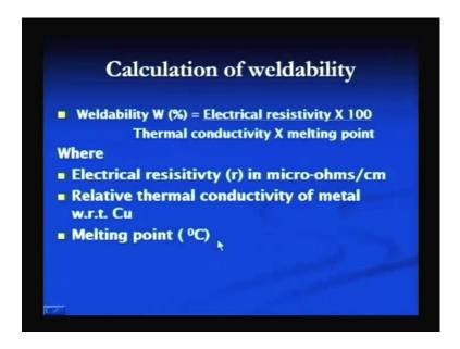
The weldability can be calculated using equation like this weldability expressed in terms of percentage like is equal to the electrical resistivity into 100 divided by thermal conductivity of the material multiplied by the melting point where electrical resistivity r in micro Ohms per Centimeter, relative thermal conductivity of the metal with respect to Copper has been quantified and it has been tabulated in handbooks can be obtained and the melting point in degree Centigrade.
