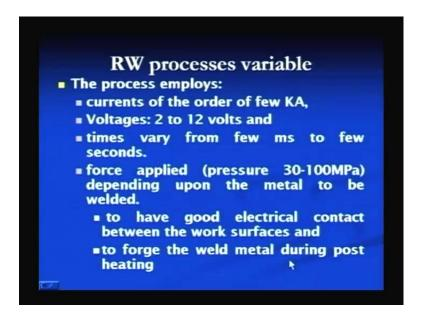
Here, if we see the variables which are to be controlled, current normally selected in the range of few kilo Amperes because these process are known as low voltage and high current. How much current is to be set? That depends upon the material to be welded and thickness of the sheets which are to be processed by the resistance welding process.
