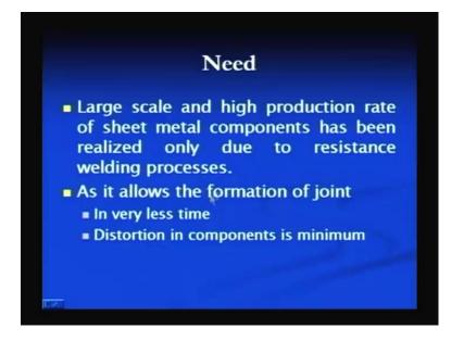
So, here we can say, for a large scale and high production rate of the sheet metal component, it is possible to use the resistance welding processes because it forms the joint in very less time. And whatever joint is formed, that is largely free from the distortion or the distortion is very less, and that is required for producing a successful joint of thin sheets by any joining process. That role is performed by the resistance welding process.
