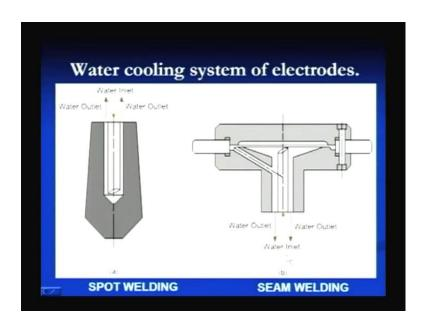
Here, water is supplied from one side and it is taken out from another side. This is the case of cooling for a spot welding purpose. If the electrodes for seam welding has to be cooled and these are used in form of rollers, and the water is supplied from one side and it is taken out from the other side to maintain the temperature of the electrodes within the same limit.
