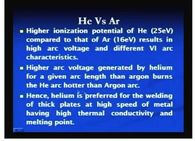
Here the argon and helium are the two extensively used shielding gases in the tungsten inert gas welding process, but we get the significant difference in their performance. What is the reason behind their performance and why the different performances are given by these gases? Those reasons we can see here.
