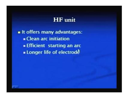
Another method is the high use of high frequency voltage process in which high frequency unit is used. This method offers many advantages like we get the clean arc initiation, no touching of the tungsten electrode to the carbon block, very efficient method and we get the longer life of the electrode with this method.
