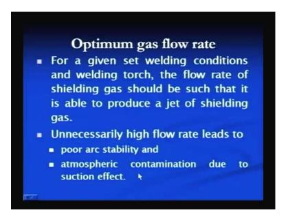
Unnecessary high flow rate should be avoided because it leads to the poor arc stability and due to the suction effect, atmospheric contamination can also be there.
