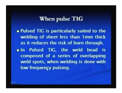
When pulse TIG is to be used, pulse TIG is particularly suited for welding of the sheets which are less than one mm thick because it reduces the risk of burn through arc, the melt through defects. In pulse TIG welding weld bead is composed of a series of overlapping weld spots when welding is done with the low frequency.
