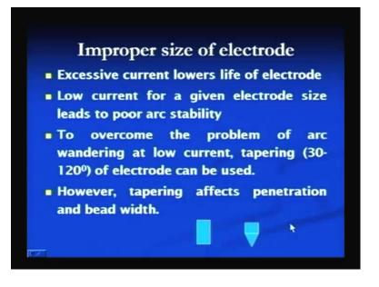
What improper selection of the electrode it can lead to or what are the problems there if the improper electrode is selected?
