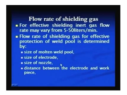
For effective shielding of the weld pool depends is governed by the number of factors like the size of the weld pool. Larger is the size of weld pool, greater will be flow rate required to cover the entire area of the molten weld pool. Size of the electrode and the size in the diameter of the nozzle, both these factors will govern the flow rate which is required to form jet of the shielding gas which can form a blanket of shielding gas around the weld pool.
