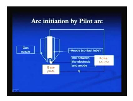
Arc initiation by pilot arc method can be seen here. A separate auxiliary power source is used here, and then arc is initially generated by using the low current between the tungsten electrode and another electrode which may be there with the nozzle. This arc is ignited initially by using the low level of current and then, it is brought to the base metal close to the base metal, so that arc between the base metal and tungsten electrode can be started.
