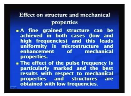
When pulse frequency and the pulse parameters are selected properly, then we get a fine grained structure. In both the cases when low and high pulse frequencies are used, but their structure which is obtained by using the low pulse frequency offers the better mechanical properties. So, effect of pulse frequencies particularly marked and best results are obtained in terms of the mechanical properties in structure with the low pulse frequencies.
