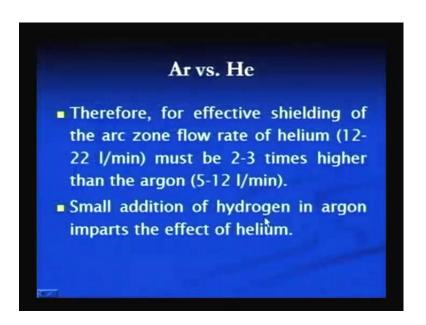
We see for effective shielding of the arc zone flow rate of the helium is around 12 to 20 liter per minute compared to that of argon which is 5 to 12 liter per minute, and this flow rate for the helium is about 2 to 3 times greater than that is required with argon. This difference is attributed mainly to the massive difference of argon and helium. A small addition of the hydrogen in argon helps to get the benefits associated with helium.
