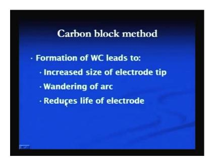
The formation of tungsten carbide at the tip is undesirable because it changes the size of the electrode tip, and it leads to the wandering of the arc and reduces the life of electrode because melting point on the tungsten carbide is somewhat lower than the pure tungsten material.
