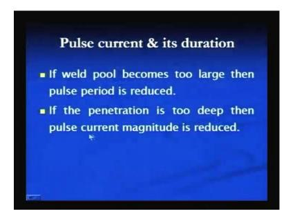
If the weld pool becomes too large, then pulse period is reduced. So, if the weld pool is of the size which is greater than the requirement, then the pulse period is to be reduced and if the penetration is too deep, then pulse current magnitude is reduced.
