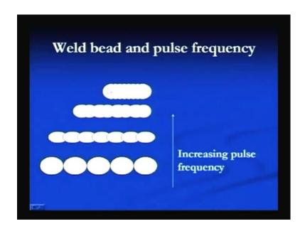
We will see in the next diagram that when the welding is done using the difference pulse frequencies, we get the different kind of spots at very low pulse frequency. The spots are just touching to each other and if we go on increasing the pulse frequency, these will start overlapping each other and normally 50 percent overlapping is used in pulse TIG welding of these spots to produce continuous and sound weld joint.
