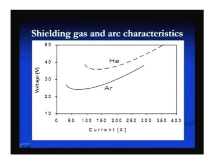
We can see here VI characteristic of the arc. For argon shows the lower arc voltage. For a given current setting here, we can say 150 ampere current, the arc voltage is somewhat 28 while for the same current setting, arc voltage is say somewhat 38. The value in both VI characteristic with both helium and argon shows the minimum arc voltage. Minimum arc voltage is around say 150 ampere with the helium and with the argon, the lowest arc voltage is at about 150 ampere.
