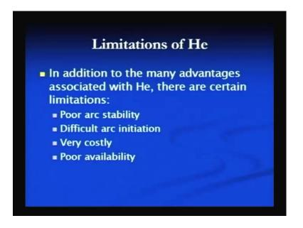
There are certain limitations associated with helium and these limitations are like poor arc stability is difficult to initiate the arc and the gas is very costly and availability is another problem. Because of these regions only, the helium is used only when very critical components arc to be welded for high reliability and high safety purpose. Otherwise, argon is invariably used for welding by the TIG process and if we compare other points related to the argon and helium.
