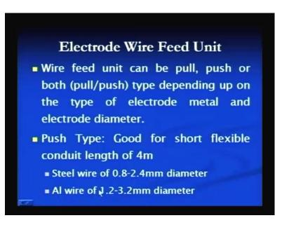
Another one is the electrode wire feed unit. Electrode wire, electrode, which is used of a required material in the different diameters is to be fed through the electrode wire feed unit in the arc region, so that smooth and continuous feeding of the wire can be achieved and a smooth and stable arc can be obtained for consistent and smooth welds.
