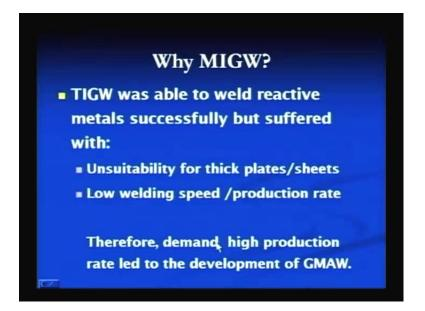
Here, the justification behind the use of the metal inert gas or gas metal arc welding process. This is what I have told you earlier that TIG was able to weld the reactive metal successfully, but it suffered with the problems, like unsuitable for thick plates, and thin, and thick sheets and the welding speed was low, which in turn produced very low production rate. And therefore, demand was there to develop new processes, which can cope with the need of the high production rate by the industry.
