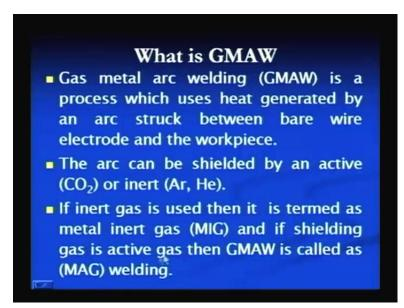
Here, for joining the reactive metals, like aluminum and magnesium, initially people struggled a lot with gas welding and shielded metal arc welding. But they were unsuccessful, because these processes, which were available in the initial stages, were not able to produce sound weld joints with, with the reactive metals. And that is why, the need was felt to develop some new processes and to cope with the difficulty in welding of the reactive metals like magnesium and aluminum.
