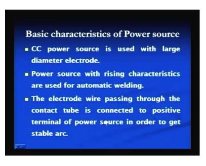
The basic characteristic of the power sources, which are used in, in, in, in the gas metal arc welding process can be of the three types. Means, all three types of the power source can be used in gas metal arc welding process like, but it is common to use the constant voltage power sources, particularly with the small diameter electrode because they offer the advantage of self-regulating arc.
