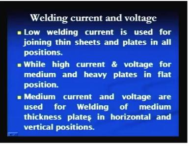
Here, low current is used when joining the thin sheets and the plates in all positions. Thin sheet welding needs special clear in terms of the heat input. Very controlled heat input is to be used for welding of thin sheets, so that the melt through or excessive heat related adverse effects can be reduced and that is possible by using the low welding current.
