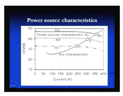
And then, the high feed rates are effective, particularly in case of the constant welding, constant voltage welding power sources. We can see, that how the constant voltage powers sources work.
