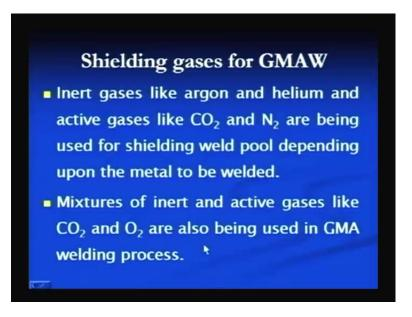
Then, shielding gases, as I have told you earlier that the shielding gas, in addition to the filler metal and the power source, also plays a significant role in successful welding of the reactive metals and the ferrous metals because these shielding gases provide the desired protection to the weld pool from the atmospheric contamination.
