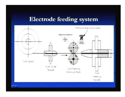
The electrode feeding system, schematically, can be seen from this diagram here. Here, is wire spool, which may be of 1 kg, which may be containing electrode wire of 1 kg, 1.12 kg or 5 kg depending upon the capacity of the spool.
