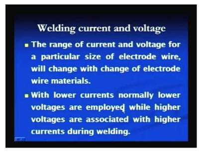
The range of current and voltage for a particular electrode size and wires, will change with the change of electrode material. Here, some of the materials can withstand up to the high current means, that they can work effectively even with the higher range of current, but that in turn, will be affected by the electrode size.
