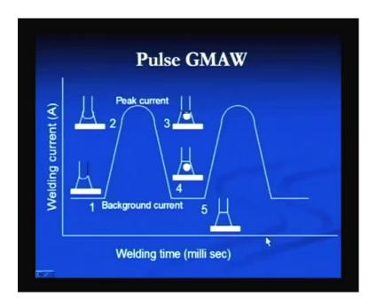
Schematically we can see that how the current varies in the pulse gas metal arc welding process. Here this is the lower level of current which is known as background current, and here the maximum current or the higher level of current which is known as peak current. Here the current is pulsed means the pulses of peak current are given at regular intervals. So, this welding current is pulsed between the background current and the peak current at regular intervals.
