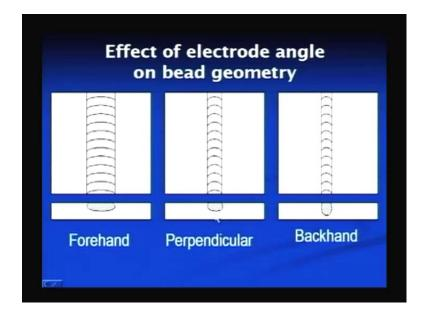
Here systematically we can see the forehand welding or forward welding. You can see here width is more and here penetration is more, and here in case of perpendicular when electrode is perpendicular to the work piece, it is an optimum one. Here this perpendicular electrode position is particularly used in automatic welding conditions, otherwise backhand or forehand welding can be used as per the needs.
