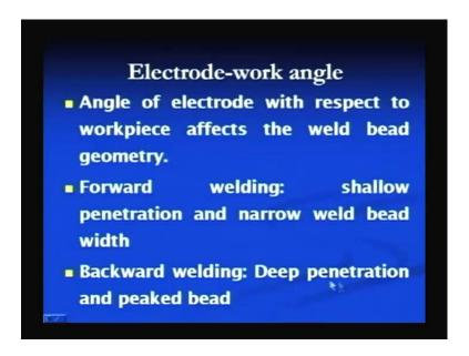
Electrode and work piece angle also affect the weld bead cross-section and the penetration, and in the forward welding when electrode is pointed towards the direction of the welding, we get the shallow penetration and a narrow weld bead width. On the other hand, when in the backward welding when electrode is pointed towards the region which has been already welded results in deep penetration and peaked bead. Here reinforcement will be high and weld bead width will be smaller one.
