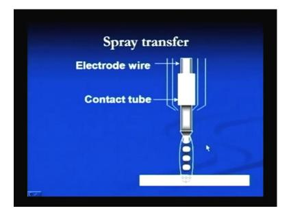
Here, schematically we can see here this is the electrode tip under the high current. The electrode, the tip of electrode, the droplets will be formed rapidly and under the affect of pinch force, it will be pinched off rapidly under the droplets will be detached even when they are of a quite small size. That gives the droplets are being sprayed from the electrode side to the weld pool, and that gives spray kind of appearance. That is why it is called spray metal transfer.
