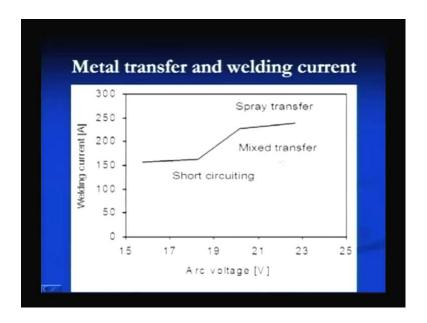
Here, spray metal transfer and welding conditions are closely related and we can see that when the current is low, we get the short circuiting metal transfer in a certain medium range, and it is mixed transfer and in the higher current side, it is the spray transfer.
