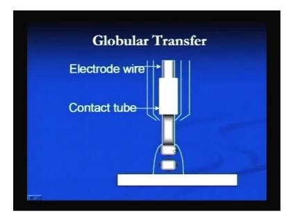
Schematically, we can see here the globular metal transfer. Here at the tip of the electrode, the molten metal droplet will be growing gracefully and as and when it attends
