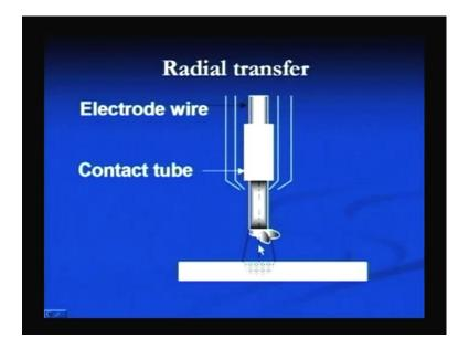
Radial transfer is another transfer due to the gases which are coming out from the weld pool side, and the various out forces leads to the movement of droplets being formed tip of the electrode in the radial directions. This leads to lot of spray or sorry, this leads to the spatter during the welding. However, it also takes place under some of the conditions.
