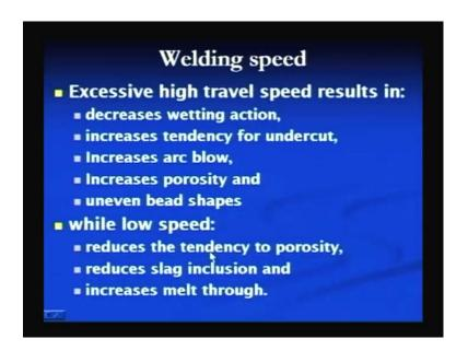
Excessive travel speed further results in decreased wetting action because of the reduced heat input, or less heat is available. And that cools down the weld pool rapidly molten metal droplets rapidly, and therefore, wetting action is decreased. Increased tendency for the undercut increases the arc blow tendency, increases porosity and uneven bead shape is produced. So, if the excessive welding speed is used, then it will further decrease the heat input, and it can create all these problems.
