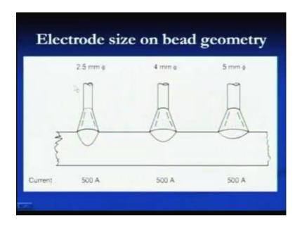
Here we can say for a given current setting if the electrodes of the different diameters are used, then how the weld bead geometry is affected? Here for 500 ampere current, the electrode of 2.5 mm diameter. Then it produces the greater depth of penetration and the limited bead width, and the bead width goes on increasing with the increase in electrode diameter, and the depth of penetration goes on decreasing with the increase in electrode diameters.
