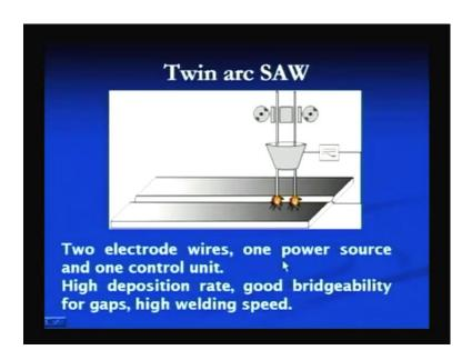
In the twin arc submerged arc welding process, we use the two electrodes, and these are powered by the same power source; the two separate wire feed units are used, and here we can see the two arcs are produced. So, in this case the two electrode wires, one power source and one control unit is used. We get the advantage of high deposition rate, good gap bridging, good birdgeability or gap bridgeability is there with this process, and we get the high welding speed because high deposition rates.
