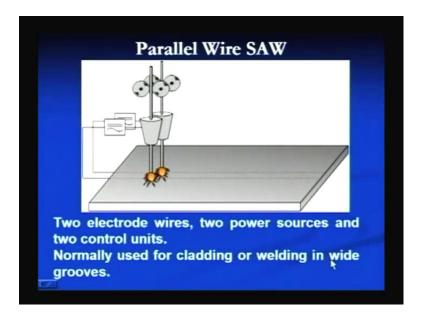
In parallel wire submerged arc welding system, the two wires move together. And in this case also these two wires move parallel during the welding, and this process uses two electrode wires, two power sources and the two control units. Normally this process is used for cladding purpose or when very wide groove is there for joining the two plates.
