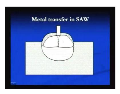
And further higher level of current helps to get the final droplets in the line of the electrode, and this is because of high pinching force that is obtained at the tip of the electrode, so that whatever droplet is being formed at the tip of electrode; that is not able to gain very large size. But before gaining a large size, it is pinched of by the presence of
