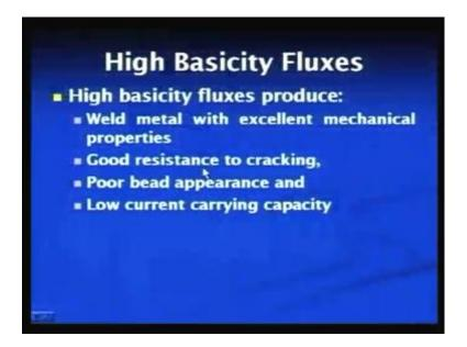
On the other hand, high basicity fluxes produce the weld metal with the good mechanical properties and good resistance to the crack propagation or resistance to the cracking; means resistance to the cracking is good, bead will not get cracked easily when basicity fluxes are used. So, from the mechanical performance point of view, the high basicity fluxes are good, but this result in low current carrying capacity and the poor bead appearance.
