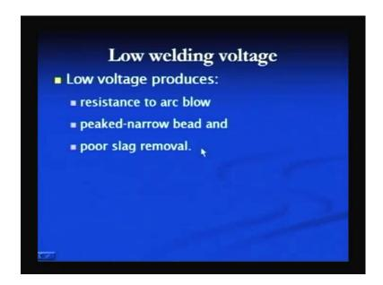
On the other hand, the low voltage setting can also create certain problems like the resistance to the arc blow peaked narrow bead is produced or poor slag removal can be there when the low voltage is set.
