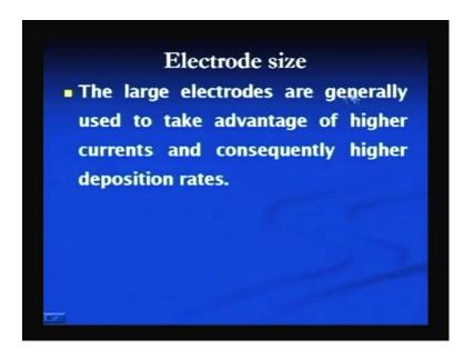
The large electrodes are generally used to take the advantage of the high current, and consequently, the high deposition rates; particularly in welding of very thick sheets where high deposition are required and high penetration is required, large diameter electrodes are selected. And also in the situations where fit up is a problem, large diameter electrodes offer the advantage of the good gap bridging capability than the small diameter electrodes.
