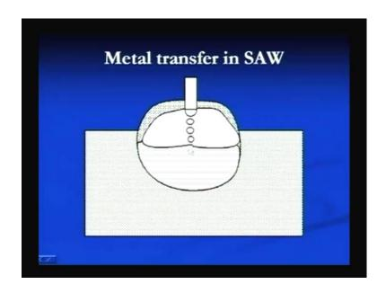
And at somewhat higher current, the droplet is detached and somewhat larger size droplets are transferred in the line of the electrode access.
