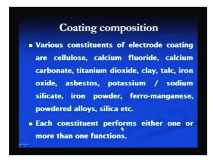
Different constituents are added in the coating materials to perform specific functions, and these coating materials are of the different types. Like the electrode coatings can have the cellulose, calcium fluoride, calcium carbonate, titanium dioxide, clay talc, iron oxide, asbestos, potassium and sodium silicate, iron powder, ferromanganese powdered alloys and silica. Each constituent is supposed to perform a specific function or more than one function.
