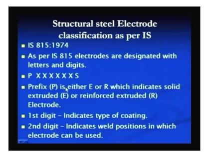
Structurally steel classification as per the Indian standard is like this. This standard is the Indian standard IS 815 was given in 1974. And as per this standard, this standard uses the letters and digits both to classify these steel electrodes. And there are the six numbers
