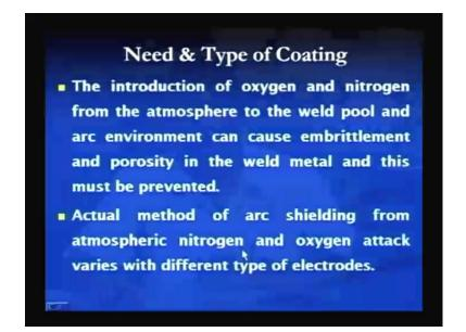
In shielded metal arc welding, the coated electrodes are used, and these coated electrodes help to produce the sound weld joints. Coatings in these electrodes are used for specific purposes; the functions are performed by these coating materials in very specific manner. So, what is the role of the coating in the shielded metal arc electrode and what are the different functions performed by the coating constraints or the coating materials; that we will see in detail one by one.
