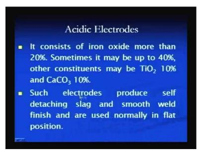
Acidic electrodes are another important kind of the electrodes; it consist the iron oxide more than 20 percent. And sometimes iron oxide can be up to 40 percent, and other constituents may be there as a titanium dioxide up to 10 percent and calcium carbonate up to 10 percent. And with such electrodes produce self detachable slag. This is important aspects, because many times it becomes difficult to detach the slag from the coating or from the weld bead.
