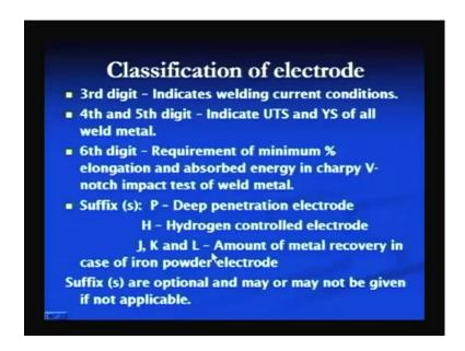
And third digit indicates the welding current conditions which are to be used, and for that particular electrode fourth and fifth digit indicates the ultimate tensile strength and yield strength of all weld metal specimen. And the sixth digit indicates the requirement of the minimum percentage elongation and the energy absorbed in charpy V notch impact test of the weld metal. So, it indicates the toughness and the percentage elongation of the weldment.
