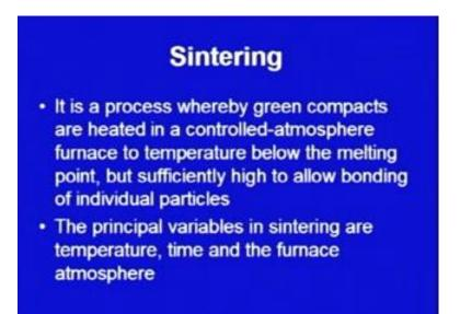
Now, coming on to the basic concept of sintering, the sintering it is a process whereby green compacts, which have been got after the process of compaction are heated in a controlled atmosphere, to temperature below the melting point, but sufficiently high to allow bonding of individual particles. As we have been discussing in the last two lectures also, that the temperature for sintering is less than the melting point of the metal.
