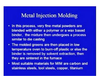
So, metal injection molding, what is this process like, in this process very fine metal powders are blended with either a polymer or a wax based binder. So, we are not going to use the metal powders as produced, but we are going to blend them with either a polymer or a wax based binder, the mixture then undergoes a process similar to die casting. The molded greens are then placed in a low temperature oven. So, the molded greens are the green compact that we get after the process of injection.
