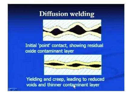
Diffusion welding is another welding process in which the components to be jointed are caped under pressure at high temperature. Initially, there is a point contact here at these locations. And gradually, when pressure is high and temperature is also high, yielding and creep at the interface takes place, which in turn increases the actual contact area, and which leads to the reduced voids and thinner contaminated layer.
