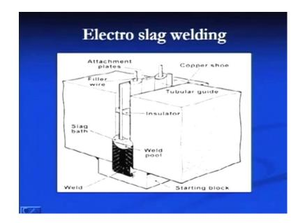
The three-dimensional diagram of the electro slag welding can be seen here. These are the two consumable electrodes at different locations; and here the copper shoes - one in this side, another can be in this side; here we have weld pool; this is the blanking plate; and this copper shoes are moved in the upward direction.
