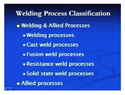
The welding and the allied processes. The welding processes are like this. The cast weld processes in which molten metal, which is generated by either flash butt welding or by any at external heat source is poured in between the faying surfaces to produce the joint. Fusion welding processes, resistance welding processes, solid state welding processes in which a metal remains in solid state and no significant heating of the metal takes place to produce the joint.
