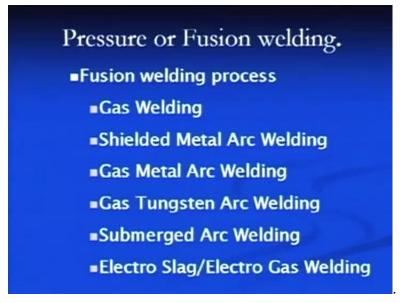
Then we will see the fusion welding processes where molten metal is produced and it is allowed to solidify freely. Then the welding processes under which such kind of conditions is produced can be like this: gas welding process, shielded metal arc welding, gas metal arc welding, gas tungsten arc welding, submerged arc welding, electro slag and electro gas welding.
