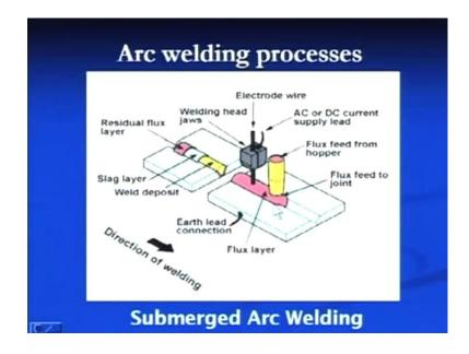
The next welding process is the submerged arc welding process, where a joint is produced by developing an arc between the base metal and a consumable electrode. And arc is submerged below the granular flux, which becomes fusible, and fusible flux melts and surrounds or covers the arc and the molten weld pool, to protect it from the atmosphere. And the molten metal is then allowed to solidify to produce the sound joint.
