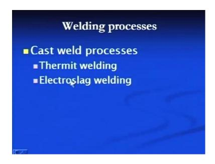
In allied processes, you will see here now, the cast weld processes are like this - thermit welding and electro slag welding. In thermit welding, molten metal is generated by exothermic reaction, and the molten metal is poured in between the plates to be joined and after the solidification we get a sound joint.
