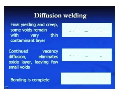
If this process continues for long, then the number of voids at the interface goes on reducing, and finally, with the continued vacancy diffusion and the removal of the oxide layer, results in very few voids at the interface. And if the diffusion welding process at high temperature and high pressure is continued for very long time, then the complete bond between the two plates can be obtained free from the voids and porosities.
