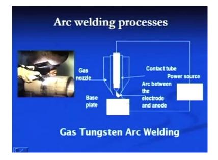
The next joining process in the arc welding processes is the TIG or tungsten inert gas welding process. In this process, the joint is produced by developing the heat between - by developing the heat from the arc, which is established between the non-consumable tungsten electrode and the work piece. And the molten pool which is generated by the arc heat is allowed to solidify to produce a sound joint.
