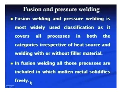
The fusion and the welding pressure welding process classification. Comments are like this: fusion and pressure welding is most widely used classification as it covers all the processes in both the categories, irrespective of heat source, and welding with or without filler material.
