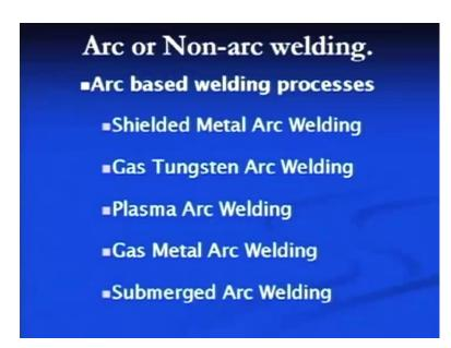
An arc welding processes are those in which electric arc is used to generate the heat desired for producing the weld joint, by melting the faying surfaces of the filler metal. These welding processes are like shielded metal arc welding, gas tungsten arc welding, plasma arc welding, gas metal arc welding, submerged arc welding.
