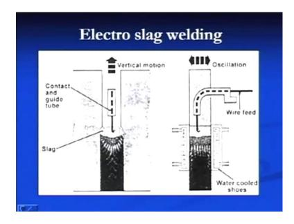
In electro slag welding process - this is a single pass welding process normally used for a jointing of thick sheets. Here, initially, an arc is established between the blanking plate
