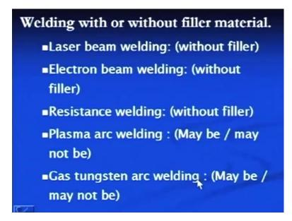
Like welding with and without filler metals can be classified like this: the laser beam welding - normally carried out without filler metal; electron beam welding - without filler metal; resistance welding - without filler metal; plasma arc welding - filler metal may be used, may not be used; tungsten arc welding - filler metal may be used, may not be used.
