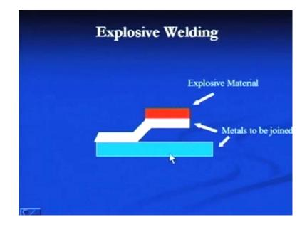
The schematic diagram or animated diagram will show that how this explosive welding works here. This is the explosive material, which is placed, and when it is detonated, the things go like this. This is know the joint at the interface is formed between the one component and the another component; and here at the interface very localized plastic deformation takes place, and that leads to the mechanical kind of bond between the two components.
