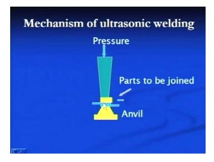
Here we will see the mechanism of the ultrasonic bonding. Here is an anvil and this is the sonotrode tip. And this is how the jointing of the two parts in ultrasonic welding takes place. Both shear stresses and the compressive stresses are held responsible for producing the joint at the interface.
