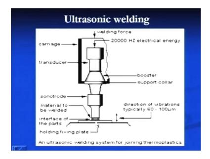
Ultrasonic welding is another process where high frequency vibrations are used to develop the bond between the two components to be joined. Here under pressure the two components are placed, and then the high frequency vibrations are provided, and that helps to generate the bond, because of the localized deformation at the interface.
