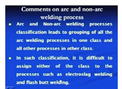
Now, we will see the comments on the arc and non-arc welding process classification. Arc and non-arc process classification leads to the grouping of all welding processes in one class and all other processes in other class; means, this if we try to classify the welding process on the basis of arc and non-arc welding processes, then all arc welding processes will come in one category, and rest of the processes will come in another category. (Refer Slide Time: 33:08)
