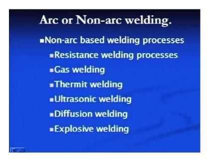
The Welding Process Classification based on arc or non-arc welding process. If you see a non-arc based welding processes are like this: resistance welding processes, gas welding, thermit welding, ultrasonic welding, diffusion welding, explosive welding.
