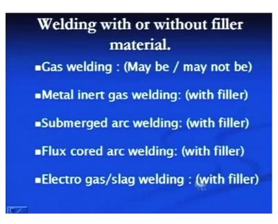
Then, we have gas welding process, gas welding process - filler metal may be may not be used; and metal inert gas welding process - filler metal is used; and submerged arc welding process carried without the filler metal, where consumable electrode acts has a filler metal; then flux cord arc welding, also with the filler metal; electro gas and electro slag welding process are performed with a filler metal.
