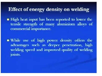
The energy density effect on the welding, we will see, at high heat input has been reported to lower the tensile strength of the many aluminum alloys of the commercial important. While the use of high energy density offers, the advantages such as deep penetration high welding speed and improve the quality of the weld joints.
