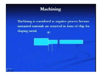
Machining is another fabrication technique in which... this is considered as a negative process, because unwanted material from the raw material or from the bulk material is removed in form of small chips for getting the desired shape of the metals.
