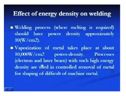
The welding process where melting is required like in all fusion welding processes, the power density should be more than 10 watt per centimeter square so as to get the faying surfaces the molten condition, and to produce the joint.
