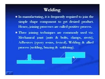
On the other hand, welding processes in which addition of the material is frequently used to get the desired size and shape. These processes in manufacturing are frequently used to join the simple shape components to get the desired product. Hence, these joining processes are called positive processes.
