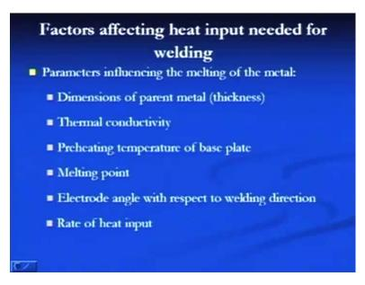
There are number of factors affecting the heat input required for welding. The parameters, which are affecting melting of the base metal, are like: dimensional parameters - dimensions of the parent metal like thickness; greater the thickness, higher the heat input required for the welding process, because heat is transferred rapidly away from the faying surfaces.
