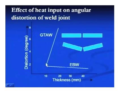
Just for example, we can see here, the effect of heat input on the angular distortion, with the increase in thickness of the plates welded by the low energy density welding process and high energy density welding process like electron beam. So, if we compare these two welding process - one of the low energy density welding process like gas, tungsten, arc welding, with high energy density welding process like electron beam welding.
