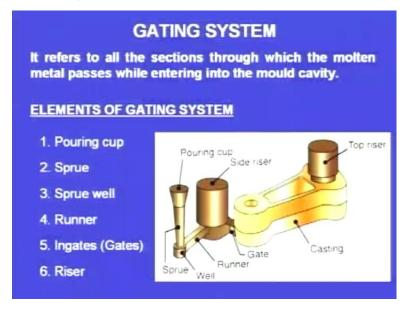
First, let us see the gating system. What is meant by gating system? Gating system refers to all the sections, through which the molten metal passes, while entering into the mould cavity. So, these are the elements of the gating system; these are shown in this diagram. The first element is the pouring cup. We pour the molten metal into the cavity, and there will be pouring cup, which is enlarged at the top and it will receive the molten metal. So, this is the pouring cup.
