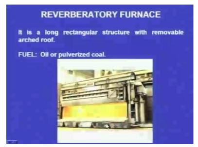
So, this is the typical appearance of a reverberatory furnace. It is a long rectangular structure with removable arched roof and the fuel used is oil or pulverized coal.
