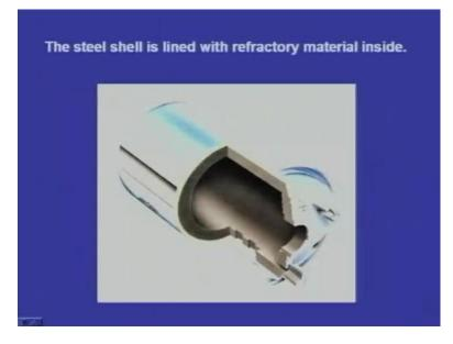
And the steel shell is lined with refractory material inside; inside there is a refractory lining. Yes, this is the cut sectional view of the rotary furnace. Inside there is refractory lining.
