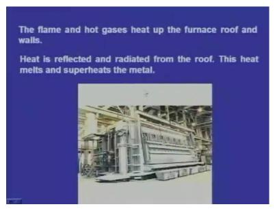
The flame and hot gases heat up the furnace roof and walls. The heat reflected and radiated from the roof will be melting and super heating the metal. Here, one thing we can notice. We use the fuel, the fuel is burning and the heat is generated, and the flame and the hot gases, they are not directly heating the charge. First they will heat the furnace
