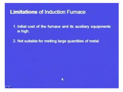
Now, let us see the limitations of induction furnace. Initial cost of the furnace and it is auxiliary equipments is high and this is not suitable for melting large quantities; only for small quantities. (Refer Slide Time: 34:53)
