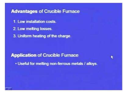
Advantages of crucible furnace: first advantage is low installation cost. After all only a crucible; we are not using any machines and low melting losses. So, here we are coming across one melting loss; what is this? In general, when we melt a metal, about five percent will be lost. If we melt 100 kgs of cast iron, we make at only 95 kgs of molten metal. So, 5 kgs of cast iron is lost. So, that is the melting loss. So, in the case of the crucible furnace, melting loss will be minimum.
