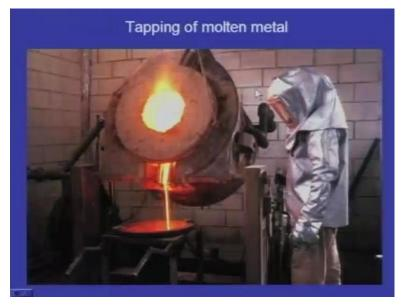
And here the molten metal is tapped from the induction furnace.
