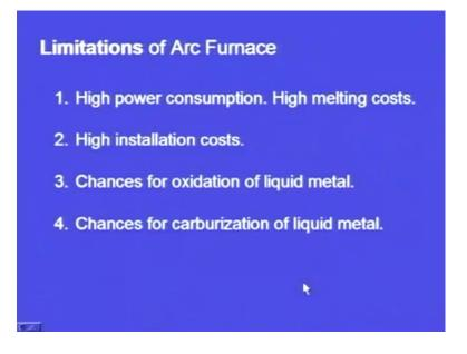
Limitations of this arc furnace: one is high power consumption. Because of this the melting cost will be high. High installation cost; the furnace itself is very costly. Chances of oxidation of the liquid metal takes place. Yes, we are sending Oxygen; this Oxygen may react with the molten metal and if the passes of the Oxygen is not controlled properly, it will be reacting with the molten metal and forms oxides. So, chances of oxidation for the liquid metal.
