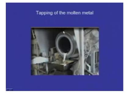
And here we can see the molten metal being tapped from the rotary furnace.
