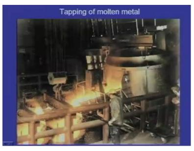
And here we can see the molten metal is tapped from the furnace.
