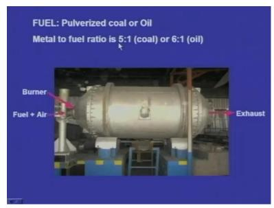
And what is the fuel? pulverized coal or oil. Metal to fuel ratio is 5 is to 1 in the case of coal. That is the metal to fuel ratio is 6 is to 1 in the case of the oil, if we use oil as the fuel. And inside the shell, there will be burner here and we are passing fuel and air this
