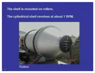
And the shell is mounted on the rollers. Here we can see the rollers; the rollers will be rotating. As these rollers are rotating, the steel shell will be rotating in the other direction. And the cylindrical shell revolves at about one revolution per minute. Slowly it will be rotating and inside the melting takes place.
