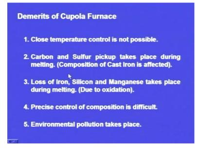
The Carbon, the permitted limit is 1.8 to 4 percent and Carbon pick up takes place means Carbon will be added to the molten metal. How? We are using coke for the combustion purpose. Coke contains Carbon. The Carbon from the coke enters into the molten metal and final content, Carbon content of the cast iron will be increasing. We are unable to control it. We are finding it difficult to control it. So, that is how Carbon pick up takes place.
