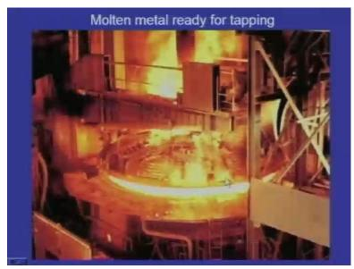
Next one, here we can see the molten metal is ready for tapping; inside we can see the molten metal.
