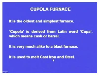
Cupola furnace is the one of the simplest furnaces ever known. The cupola is derived from the Latin word cupa which means cask or barrel, barrel or a shaft; it looks like a shaft and it looks like a blast furnace. Of course blast furnace is very big and the principle of operation and the purpose are different, but appearance wise it resembles the blast furnace and it is used to melt cast iron and steel. Let us see the construction details of the cupola furnace.
