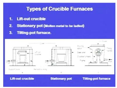
There are three types of crucible furnace: one is lift-out crucible; second one is stationary pot in which molten metal has to be ladled; third one is tilting pot furnace.
