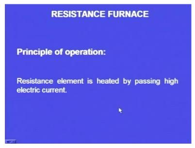
The principle of operation is resistance will be there in the furnace; when we pass electricity through the resistance, the resisting element will be heated up and this heat will be utilized to melt the charge. So, that is the principle.
