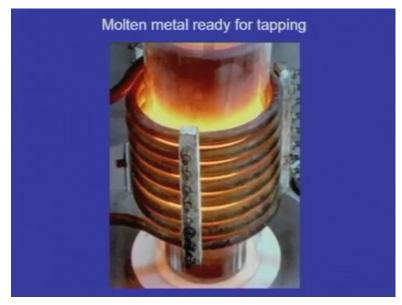
Here, we can see the induction furnace in operation. So, this is the coil and this is the crucible. And inside the crucible, we have kept the charge. So, heat is generated and the charge inside the crucible is melting.
