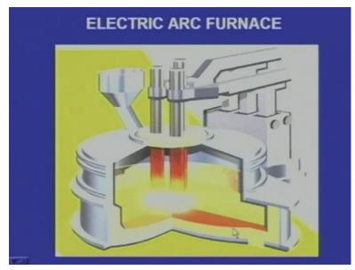
So, this is the cut sectional view of arc furnace. Here we can see the electrodes; graphite electrodes are there. And this is a shell and inside there is a charge, metallic charge, which we want to melt. The power supply is connected between the electrodes and the charge, and we strike these electrodes and sparks are created, and that continues into arc. And because of this arc, the molten metal is prepared; the charge melts. So, this is the principle of the electric arc furnace.
