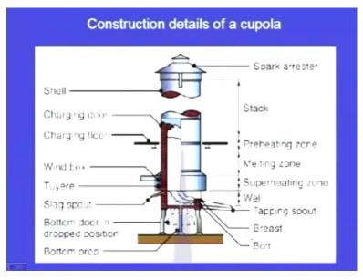
So, this is the construction details of the cupola furnace. Here we can see the furnace. These are the different components of the furnace. Let us study these different components of this cupola furnace.
