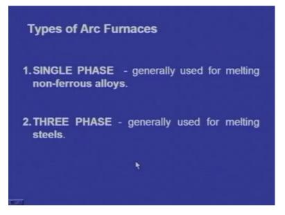
Types of arc furnaces: There are two types of arc furnaces: one is single phase and other one is the three phase. The single phase arc furnace is generally used for melting nonferrous alloys and the three phase arc furnace is generally used for melting steels.
