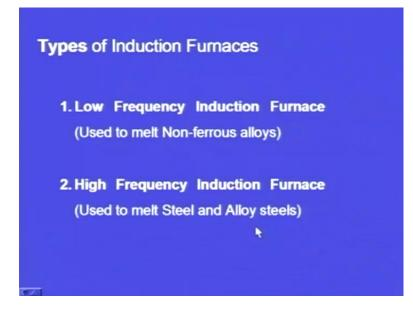
Types of induction furnaces: There are two types: one is low frequency induction furnace and this is used to melt non-ferrous alloys like Aluminum, Copper and so on, and the other type is high frequency induction furnace and this is used to melt steel and alloy steels.
