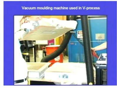
Here we use a vacuum moulding machine. So, this is the vacuum moulding machine. We can see this is a very sophisticated machine and here we can see the strong polymer will be covered, and this is the machine which is used in the V process. Here we can see arrangement for applying vacuum. Let us see the step by step involved in this V process. First, say we have to use a precision pattern. The pattern should be of extreme precision and no allowances are required.
