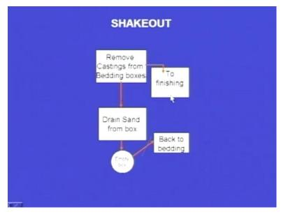
Next one is shakeout. After solidification is over, we have to remove the casting from the bedding boxes and the sand will be broken. The sand has to be drained from the boxes and the boxes will be empty. Again they will be going to the bedding and here the castings will be going for finishing the operations. So, this is the shakeout.
