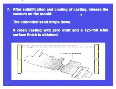
After solidification and cooling of the casting, release the vacuum on the mould.
