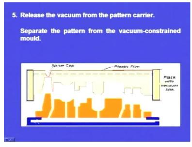
Vacuum, here we have applied at the pattern carrier. This vacuum has enabled us so that the polymer sheet will be occupying exactly over the pattern. So, that is the purpose of applying the vacuum here. We have applied vacuum at another place that is in the flask; this vacuum has helped us to hold the sand tightly inside the flask.
