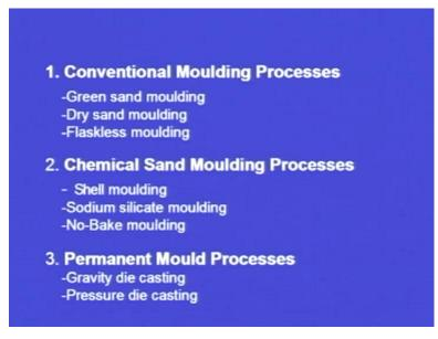
We have seen the green sand moulding, we have learnt dry sand moulding, and we have learnt flaskless moulding. These constitute conventional moulding process.
