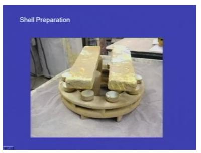
So, we can see, a shell is created over the pattern assembly. So, this is the pattern and these are the risers.
