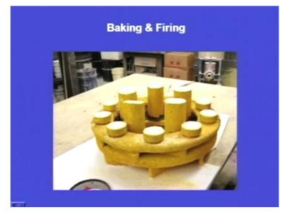
Yes, when we bake and fire, the shell looks like this. This is the shell and inside the EPS pattern has been evacuated. Now, we can see the shell; the bake and fired shell. (Refer Slide Time: 29:59)
