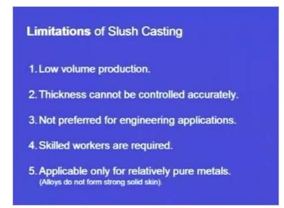
These are the limitations. Low volume production and thickness cannot be controlled accurately. Thickness can be control arbitrarily and this is not preferred for engineering applications. Only this is applicable for art items and for this skilled workers are required because we pour the molten metal and when the outer shell solidifies, when the inner part is in still liquid state, that time we have to pour out the liquid metal and for that skilled worker is required.
