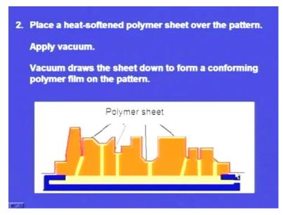
Next, we have to take a strong polymer and that strong polymer we have to soften by heat. After softening the polymer sheet by heat, we have to place it over the pattern like this. Here we can see this red color one; so, that is the strong polymer, polymer sheet. And at the end, we have to seal it.
