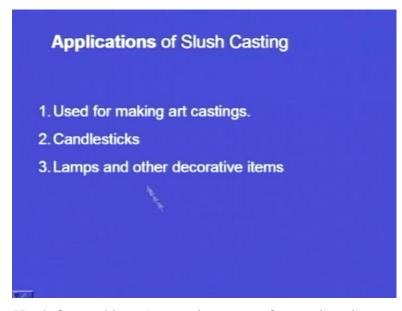
Applications: Used for making Art castings; not for engineering applications; for example, candlesticks. These are made by slush casting lamps and other decorative items. These are made by slush casting.
