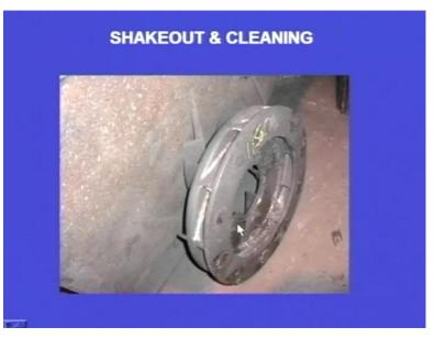
So, this is the final casting that we have obtained after solidification and after shakeout. (Refer Slide Time: 32:19)
