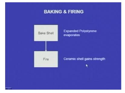
Next one is baking and firing. The expanded polystyrene pattern will be evaporating while we are baking. Yes, we will place the pattern assembly in an oven and we will bake it; we will dry it. Next one, it will be fired. The ceramic shell will be getting strength when we fire it. So, this is about baking and firing.
