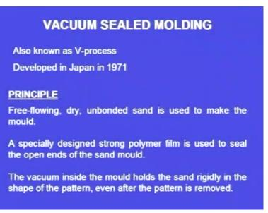
This process is also known as V process. This was developed in Japan in 1971. What is the principle involved in this vacuum sealed moulding or V process? Here, free flowing, dry and unbounded sand is used to make the mould.
