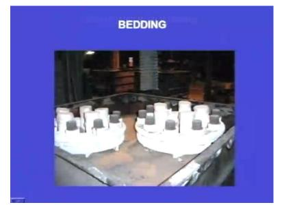
Yes, this way we have kept. This is one shell; so, this is one shell. These shells, we have kept over this above the sand. Then we pour the molten metal.
