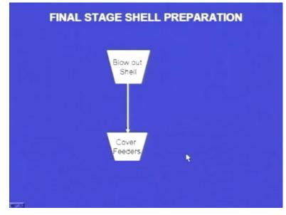
Next one is final stage of the shell preparation. So, we have heated the pattern in an oven. The EPS pattern has evaporated and it has gone. It has escaped from the shell. Still small traces of the pattern may be inside. So, we have to blow out. We send pressurized air through the shell. Then, any small amount of pattern that is left inside the cavity will be thrown out will be coming out. Next one is the feeders. Feeders means this. Risers we will be covering.
