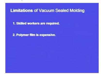
And this process has got some limitations. Here we have to apply vacuum and this vacuum should be controlled very carefully. It the vacuum is not controlled very carefully, the sand which is held rigidly inside the moulding flask will be collapsing at any stage; that may be a failure. So, for this, we require skilled workers. And the polymer film which we are using is expensive. So, these are the limitations of the vacuum sealed moulding process.
