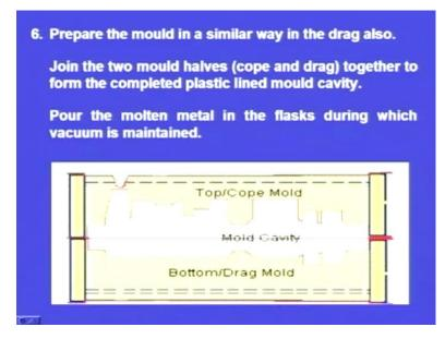
Next one, prepare the mould in a similar way in the drag box also. So, far we have seen preparing the mould using this polymer sheet and vacuum in the cope box, that is the upper moulding box. Now, we have to prepare the mould in the drag box also, that is the lower moulding box. So, this is the drag box; the lower moulding box. This one also, in the same way, we have to prepare using vacuum and polymer sheet.
