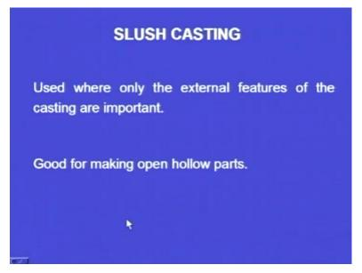
Slush casting: This is used where only the external features of the casting are important and this is good for making hollow parts.
