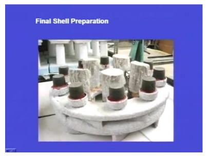
Yes, these are the feeders. These feeders will be covered. So, this is the final shell preparation.
