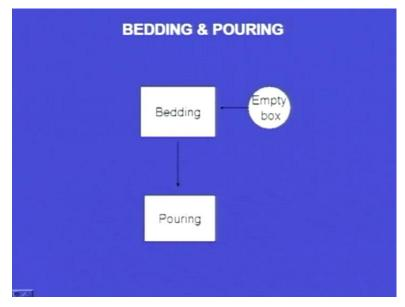
Next one bedding and pouring. So, we have to place this mould, the shell in a box where there is sand; may be sometimes we may pour more than one box or more than one shell. So, all these shells we have to place in a moulding box. So, that is the bedding. Then, we pour the molten metal into the shells.
