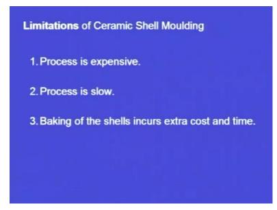
Limitations of this ceramic shell moulding: The process is expensive. The pattern material that is the EPS, the expanded polystyrene, is expensive. We have to give slurry coating. We have to give stucco coating. These are expensive. We have to keep them in ovens for baking; that makes the process expensive.
