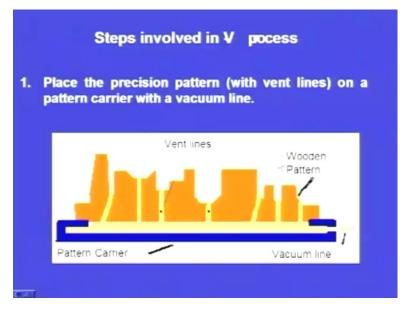
And this pattern has got some vent holes. We can see so many holes are there. Here one hole, here one hole. So, these are the vent holes for the pattern and this pattern we have to place it on a pattern carrier; so, this is the pattern carrier. So, over this pattern carrier, we place the pattern and this pattern carrier has got a vacuum line through which we can apply vacuum.
