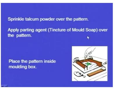
Next one, we have to sprinkle talcum powder over the pattern to get a fine finish over the cavity surface. Next one, apply parting agent, which is the Tincture of Mould Soap over the pattern. So, this helps us for parting purpose, so that the plaster will not be sticking to the pattern.
