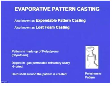
Evaporative pattern casting, this process is also known as expendable pattern casting. This process is also known as lost foam casting. And here, the pattern is made up of polystyrene or the Styrofoam. Let us see the step by step procedure in this evaporative pattern casting.
