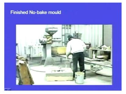
Here the mould is prepared and here, we can see the mould for even from its appearance, we can see it has got good surface finish and also, it offers good dimensional tolerances.
