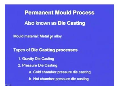
So, this permanent molding process is also known as die casting. Permanent molding process is also known as die casting and the mould material is metal or alloy. There are two types of die casting process. One is gravity die casting in which there will be a set of
