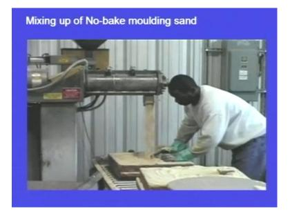
We can see here this no-bake molding sand is prepared and because this urethane reacts with silica sand very quickly, within few minutes it will be hardened. So, the mould should be done quickly. Not that we can mix the sands for some time and we can leave it just like that for some time, because it will be hardened. So, once we prepare the sand, immediately we should prepare the mould.
