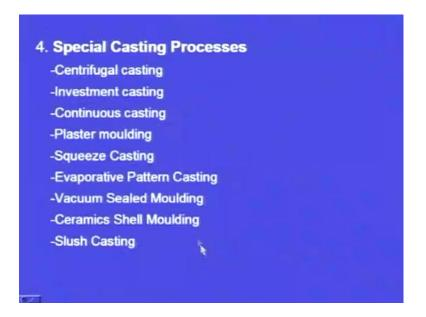
Fourth one is special casting processes and among the conventional molding processes, green sand molding is widely used. In fact, our ancestors have been using this green sand molding, and the molding medium is not costly and any big component can be
