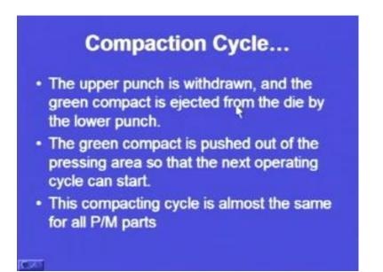
The upper punch is withdrawn, and the green compact is ejected from the die by the lower punch. Now, step three we can see the upper punch is withdrawn, and the green compact these black portions are the product that we are making is withdrawn with the help of the lower punch. The green compact is pushed out of the pressing area, so that the next operating cycle can start.
