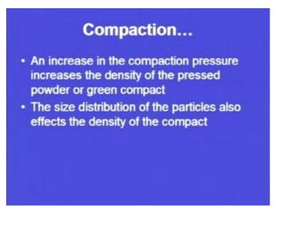
So, as we have seen that the strength of the green compact is also important for further processing of the green compact. So, now the third point to be considered in compaction is, an increase in the compaction pressure increases the density of the pressed powder or the green compact. So, if we increase the compaction pressure, the density of the pressed product or green compact will improve. So, increasing the compaction pressure will
