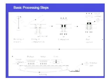
Now, this gives a line diagram of the basic processing steps, so we can see that this is the blending of the powders, so this is one shape Y shape kind of all equipment in which we put the different metals, whose powder have to be made the powders have already been made, we put them for blending processes here. So, different powders will be put here and this will be rotated as is shown in the diagram, this is the rotation taking place. So,
