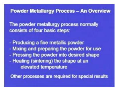
Now, we come onto the powder metallurgy processes, so already till now we have seen, that we can make metal powders using different processes, and there are certain hazards related to the metal powders. Before that we have seen that metal powders of different metals need to blend it together, to give the final mechanical as well as the physical properties to the powder metallurgy part.
