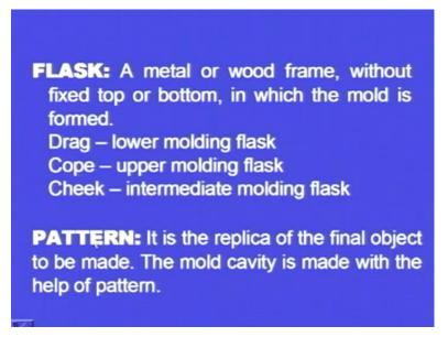
And the first one is the flask. It is a box made up of metal or wood. As I already told in the beginning, the principle of metal casting is, we will create a cavity in a compacted sand medium or any moulding medium and the cavity, cavity's shape will be similar to that of the component, which we will be manufacturing. So, this compacted sand medium will be made within this flask.
