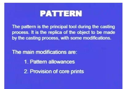
The pattern, so the pattern is the replica of the object to be cast. So, as I have already told, it acts as the model to create the mould cavity. So, whenever we want to cast a particular component we have to create a cavity whose shape is similar to that of the
