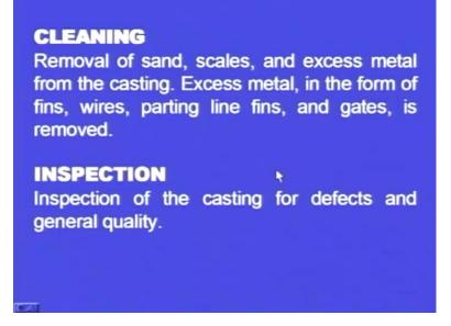
Next one, cleaning. After we pour the molten metal into the cavity, after sometime the casting will be solidified and so much of sand will be sticking to the casting. There will be so many scales and there will be, extra metal projections will be there. And we have to remove the sand, we have to remove the scales, we have to cut off the excess metal scales. So, this process comes under cleaning.
