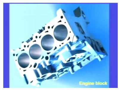
This is another engine block where we can see four cylinders. This complex shape is manufactured by metal casting.
