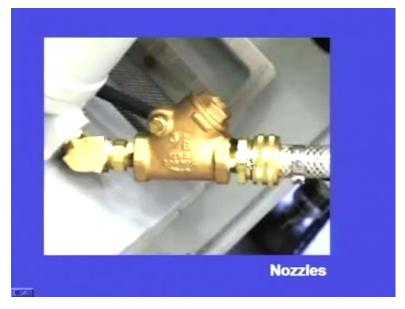
These are the nozzles. These nozzles are manufactured by metal casting.
