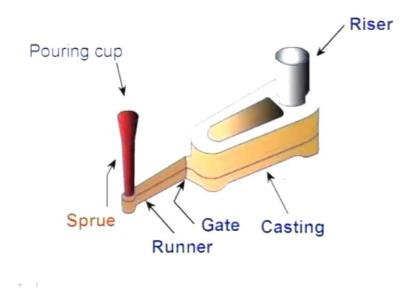
And this is another casting. Of course, this is shown without moulding boxes. So, this is the pouring cup, this is the Sprue, so this is the Runner. Initially, the molten will be pour in the pouring cup, then it will be passing through the sprue and it will be reaching the choke. And finally, it will be reaching the runner and finally, it will be reaching the casting.
