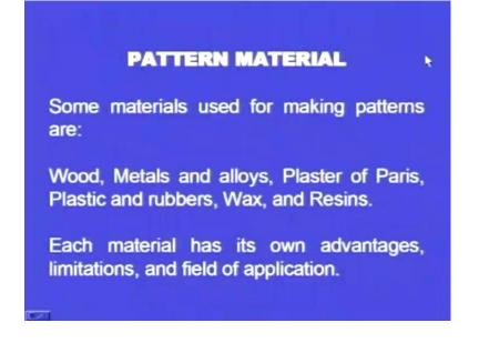
And what about the pattern material? Most of the times the pattern material is wood. In some cases it is metal, sometimes it is made up of alloy and Plaster of Paris is also used, where we achieve good dimensional accuracy and also good surface finish. We use plastic and rubber, we also use wax where we get excellent surface finish and also, we use resins. So, these are all the pattern materials.
