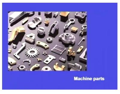
And we can see so many components, small components, tiny components, complex components, all these components are manufactured by metal casting. And these are, whatever I have taught is only few examples, there are many more examples where there are many components, which can be manufactured by metal casting.
