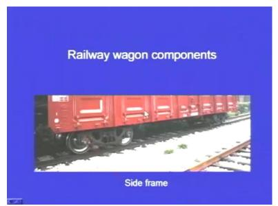
And metal casting technique is used in railway components. And here, we can see, this is a goods wagon and here we can see one important component, that is, the side frame, which is lying about two axles, railway axles, and this is the side frame. This side frame is manufactured by metal casting. I will show you this side frame in a magnified view.
