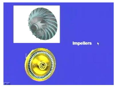
These are the impellers. These are manufactured by metal casting.
