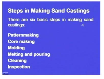
And let us see the steps in making sand casting. There are six basic steps involved in making a sand casting. One is pattern making, second one core making, next one moulding, melting and pouring, cleaning and finally, inspection.
