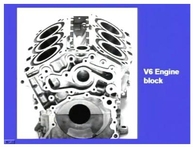
This is an engine block, V6 engine block. Here, you can see, three cylinder this side, three cylinders this side and this whole thing comprises an engine block. This is manufactured by metal casting.
