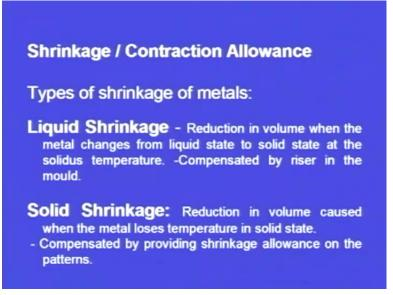
Shrinkage allowance or this is also known as contraction allowance. What is this shrinkage allowance? Yes, when we make a casting during solidification, it undergoes shrinkage. If we want a particular size and if we make the pattern exactly as the size of the required casting and during the pouring stage, during pouring and during solidification the metal solidifies, it undergoes shrinkage.
