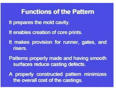
And what are the functions of the pattern? First function is, it prepares the mould cavity. Whatever component or whatever shape we are going to make, we use the pattern of a similar shape. And when we keep the pattern inside the moulding boxes and we ram the moulding sand, we compact the moulding sand. After compaction is over we remove the pattern and there will be a cavity whose shape is similar to that of the casting, that we are going to make. So, it prepares the mould cavity.
