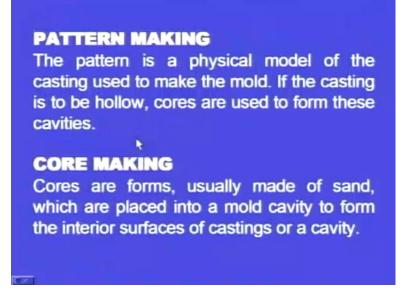
First one is, pattern making. What is this pattern to make a casting of particular shape? What we do is, we create a cavity in the sand medium. The shape of the cavity will be similar to that of the casting, which we are going to make. So, to make the cavity we have to use a model. This model is known as the pattern. So, first we have to create the pattern.
