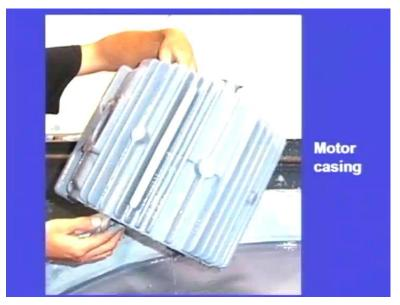
This is a motor casing. This is manufactured by metal casing.
