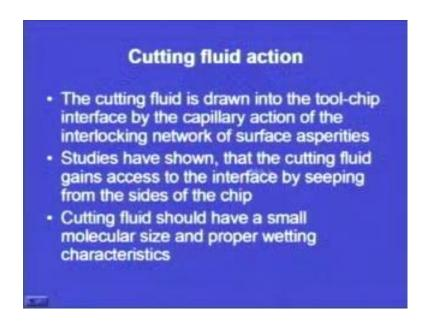
Now, how the cutting fluid acts or the cutting fluid action - the cutting fluid is drawn into the tool chip interface. There is a tool chip interface, already we have seen, by the capillary action of the interlocking network of surface asperities. So, there are some surface asperities in this meeting part, and in the surface asperities by the capillary action the cutting fluid is drawn into.
