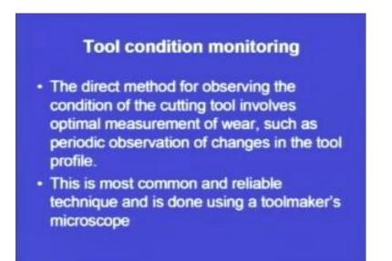
Now, we need to monitor the tool condition. We have seen that the tool is subjected to a number of testing conditions. Now, when the tool is under those conditions, under highly localized stresses, under high temperature, it is that the chip is rubbing against the tool, and the tool is rubbing against the work piece. So, under all these testing conditions, the tool wear is going to take place; the tool wear is going to depend upon a number of parameters.
