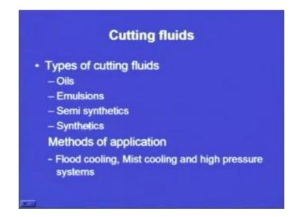
Now, what are different types of cutting fluids? Now, different types of cutting fluids can be oils, these can be emulsions, these can be semi-synthetics, these can be synthetics. So, depending upon the different types of requirements, we have to choose among different types of cutting fluid. So, we have a wide variety of cutting fluids that are available and depending upon our requirement we will choose any of these.
