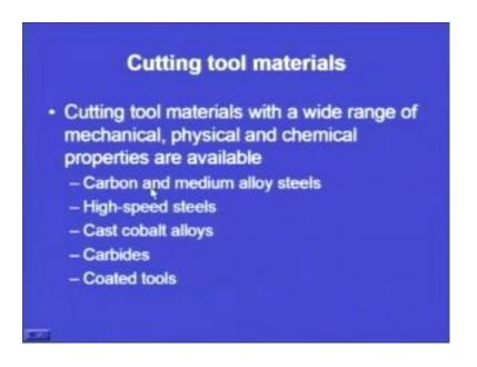
Now, cutting tool materials with a wide range of mechanical physical and chemical properties are available. So, there are number of cutting tool materials available. What are these different types of cutting materials? These are in order of how they have found their significance.
