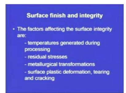
Now, surface finish and integrity, we will continue the factors affecting the surface integrity. So, what are the various factors that affect the surface integrity? These are the temperatures generated during processes or the temperatures generated during processing, these will depend on the residual stresses; these will also depend on the metallurgical transformations; moreover, they will depend upon the surface plastic deformation tearing and cracking.
