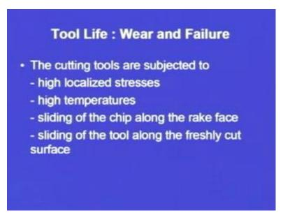
Now, tool life has two important points that is wear and the failure. So, wear is anyhow going to take place, whenever suppose, one particular example that comes to my mind
