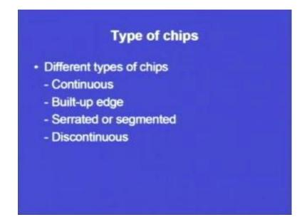
Now, already we have discussed, what are the different types of chips, just I will briefly summarize, the different types of chips that are formed are continuous chips, chips with built up edge, serrated or segmented chip, and discontinuous chips. So, now we will discuss each one of these types under what conditions this types of chips are formed, and what is the influence on the surface finish etcetera?
