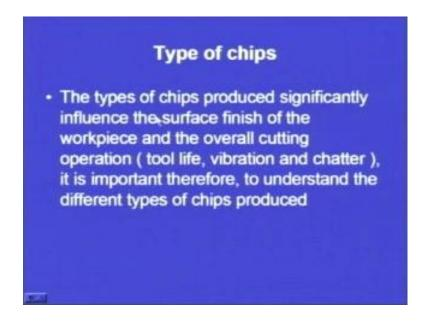
Now, types of chips, the types of chips produced significantly influence the surface finish of the work piece. Now, previous lecture also we have seen now also we have seen in the limitations also of the machining operation that the type of chip has certain bearing on the surface finish of the final product that we will get. So, how is that influencing, that is influencing, when the chips that are formed are continuous in nature.
