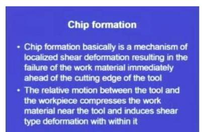
Now, chip formation basically is a mechanism of localized shear deformation. So, deformation is taking place here also, and it is the localized shear deformation. So, chip formation basically is a mechanism of localized shear deformation, resulting in the failure of the work material immediately ahead of the cutting edge of the tool. So, suppose, this is the material that we want to machine, this is suppose the cutting tool, our localized area just ahead of the cutting tool.
