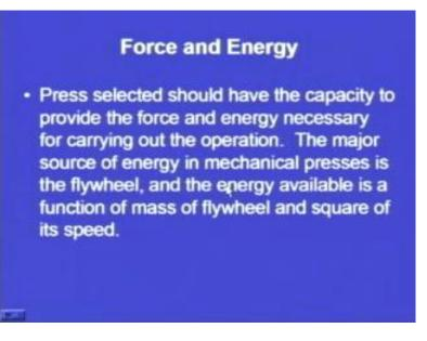
Now, force and energy requirements. This is another important parameter of acting the selection of a press. Press selected should have the capacity to provide the force, and
