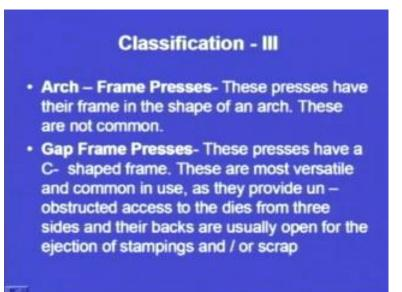
So, arch frame presses. These presses have their frame in the shape of an arch. So, the frame has a shape of an arch which we will see in the subsequent slide, where we will see the diagram. These are not very common. So, arch frame presses, although they are in use, but are not the most common presses that are used.
