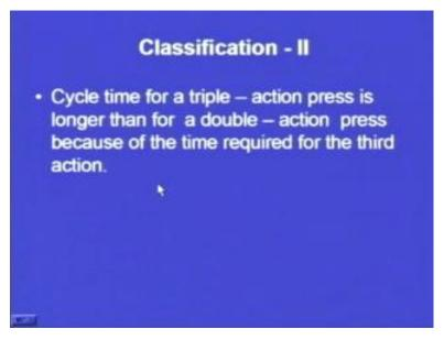
Cycle time for a triple action press is longer than for a double action press because of the time required for the third action. So, this is quite normal that when we have to perform another operation, so the cycle time that will add on the complete cycle time, the cycle time or that amount of time that is required using a triple action press is more than a double action press. Coming on to the third important classification that is on the basis of frame and construction.
