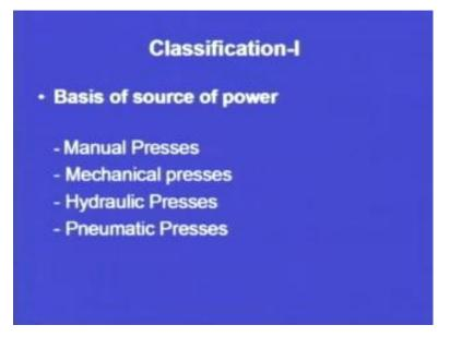
So, already I have told either the presses can be hydraulically operated, or they can be pneumatically operated. They can be mechanical presses or these can be manual presses. So, depending upon the source of power, four different classifications have been there. How the presses are operated, or what is the source power for the press. So, we have seen that it can be manual mechanical hydraulic or pneumatic press.
