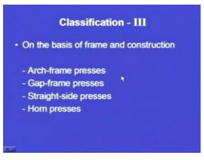
So, on the basis of frame and construction, we can have different types of presses. What are those different types of presses? There are arch-frame presses, gap frame presses, straight side presses and horn presses. So, we will try to understand these different types of presses with the help of a very simple diagram.
