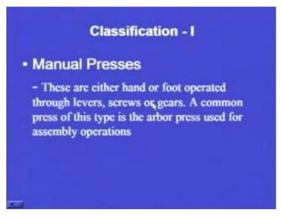
Now, what is the manual press or what are the different manual presses? Now, manual presses are either hand or foot operated through levers, screws or gears. So, manual as
