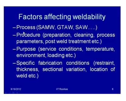
So, as far as the process is concerned, a given material can be of very good weldable, can be of very good weldability for by a particular process. But, may be poor by other process that is why, it is important to consider, which process is being used for developing a weld joint. For example, aluminum welding is found difficult to weld by the gas welding and shielded metal arc welding process, but when it is welded by the GTA or GMAW processes then it can be welded easily.
