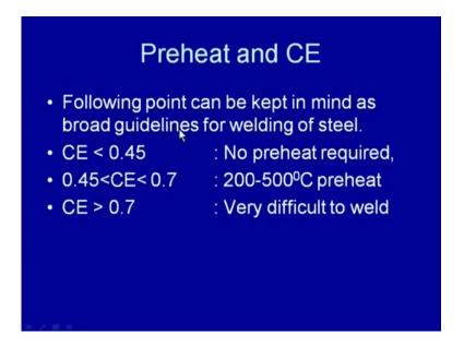
As a guideline, the following points can be kept in mind to avoid the cracking in the welding of the steel. And so that the satisfactory weld joint can be developed say, if the carbon equivalent is less than 0.45, as calculated using above equations then no preheating is done. But, if the carbon equivalent is in the range of 0.45 to the 0.7 then preheating of 200 to 500 degree centigrade is done and if it is more than 0.7 then it is found very difficult to weld.
