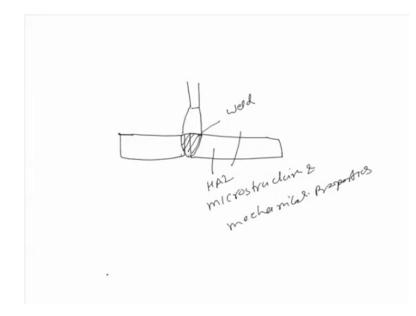
So, to understand this we will be starting with this schematic diagram, which we will be showing that, if we are required to develop a weld of a given metal, then heat is applied to melt the faying surfaces by fusion welding processes. So, the application of the heat using the suitable heat source, whether it is arc or the flame will be bringing the faying surfaces to the molten state. So means, basically we will be applying the heat to melt the things and develop a weld.
