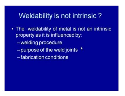
Weldability of the metal is not an intrinsic property because it is governed by the many other factors related with the welding like the welding procedure, which is being used affects the weldability in a big way. Because, ranging from the cleanliness, edge preparation of the weld, welding process, the preheating, post weld treatment, all these factors significantly affect the quality of the weld and the associated cost, and the efforts required.
