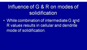
While a combination of the intermediate values of the G and R results in the cellular and the dendritic mode of the solidification.
