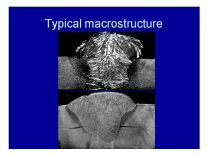
Like though first, we have the planar solidification because the G by R ratio is found high near the fusion boundary then we have the cellular structure slightly away from the fusion boundary then it is columnar, dendritic and finally, equiaxed at the weld center. So, because of the changing G by R ratios, which is very high at the fusion boundary and very low near the weld center, we come across all these 4 modes of the solidification especially, in the weld zone.
