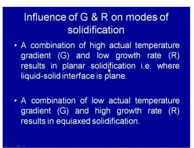
So, as far as G and R are concerned, a combination of the high means, high value of G and low R results in the planar solidification and a combination of the low G and high R results in the equiaxed solidification.
