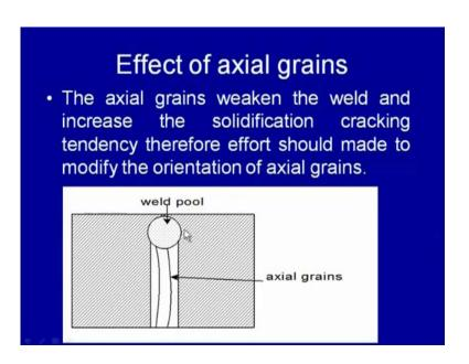
So, we can say this is the weld pool and the grains which are growing like lengthwise, they are axial grains and the grains which will be growing perpendicular to the fusion boundary, which has been of the base metal, which has been melted, they will be developing the columnar grained structure. So, axial grains weaken the weld and increase the solidification cracking tendency and therefore, efforts should be made to modify the orientation of the axial grain.
