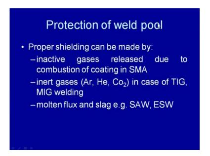
Similarly, the slag metal reactions will also be occurring due to the entrapment of slag inclusions will be developed. But, all these reactions will be governed by that, how effectively the weld pool is being protected. So, the processes which provide very effective weld pool, they will be producing the cleaner weld. So, the weldability of the metal will be better and because of this, the weldability of the metal becomes sensitive to
