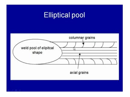
If we see the welding speed and the heat input, appreciably affect the orientation of the
