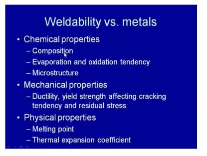
So, the chemical composition of the weld metal affects the weldability significantly like the presence of certain alloying element in the metals tends to evaporate or intends to get oxidized in the arc environment. And that will be leading to the change in chemical composition of the weld metal or it will be increasing the, due to the oxidation tendency there will be increasing the oxide inclusions in the weld metal.
