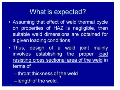
So, this is how we if we try to identify, the load resisting cross sectional area of the weld joint in terms of the throat thickness and the length of weld, which is to be deposited. Say the approach for determining the throat thickness and approach for determining the throat thickness for the butt weld is found to be different from that of the fillet weld.
