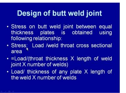
To design the butt weld joint, the stress on the butt weld joint between the equal plate thickness is obtained using this relationship, where the stress is equal to the load divided by the weld cross sectional, weld throat cross sectional area. Where and further the load divided by weld throat thickness multiplied with the length of the weld into the number of weld.
