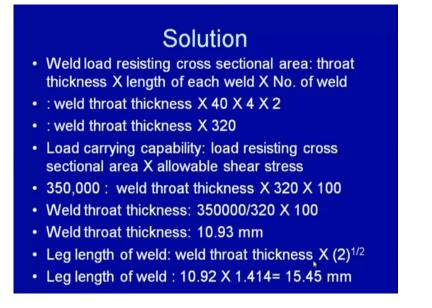
So, solution goes like this where we basically try to see that the how applied how to calculate, the load resisting cross sectional area. So, that it can sustain the external load which is being applied. So, weld load resisting cross sectional area is obtained from the throat thickness of the weld multiplied by length of the each weld and the number of welds, that are being made.
