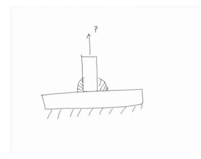
So, for given loading conditions basically, the weld dimensions are identified in terms of the weld throat thickness and the length of the weld. So, thus the designing of the weld joint mainly involves the establishing, the proper load resisting cross sectional area of the weld. And this load resisting cross sectional area of the weld is established in terms of the throat thickness of the weld and the length of the weld.
