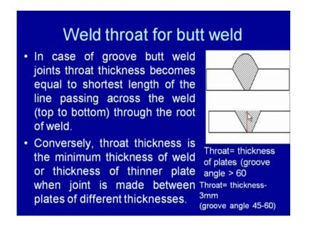
In case of the butt weld groove, but weld the joint throat thickness becomes equal to the shortest length of the line passing across the weld through the root, so the line which is passing the shortest line, which is passing through the weld and through the root. So,
