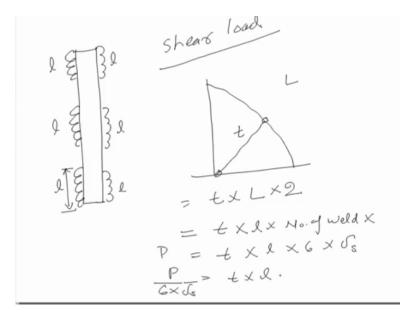
So, to identify the load resisting cross sectional area for fillet weld basically, we determine the throat thickness, which is obtained from the shortest distance of the line, which is passing through, the root and the face of the weld. And so this is the throat thickness say t and the length of the weld. So, length of the weld say if it is L then t into L gives the load resisting.
