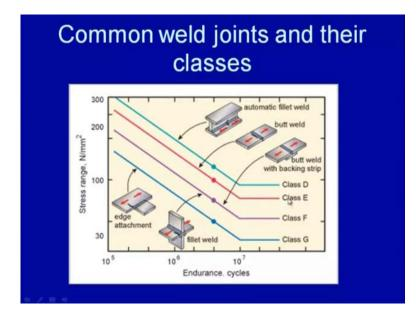
For developing the weld joints for applications, where fatigue loading takes place on the weld joint, it is desired to classify the weld joints under the different classes, which indicates the severity for which a weld joint will be subjected. So, higher is the class greater will be the severity of the stress conditions and lower will be the fatigue life of the component.
