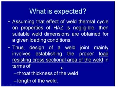
So, assuming that the effect of weld thermal cycle on the H A Z is negligible, then the suitable dimensions of the weld are obtained for the given loading conditions. So, primarily in the design of designing of the weld joint, it is identified what will be the dimensions of the weld load resisting cross sectional area. So, that it can sustain the service load.
