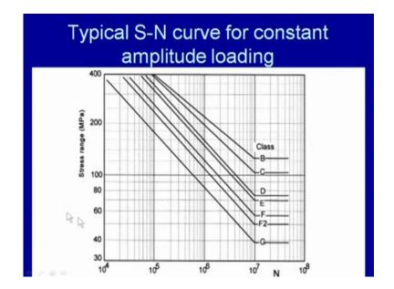
So, if we can see here, further this diagram B will be considered in the higher class and C D E F F 2 G will be considered in the lower class. So, lower is the class of the weld lower will be the allowable stress range and this allowable stress range will be used for determining, the load resisting cross sectional area for the fatigue joint for designing the weld for fatigue joint.
