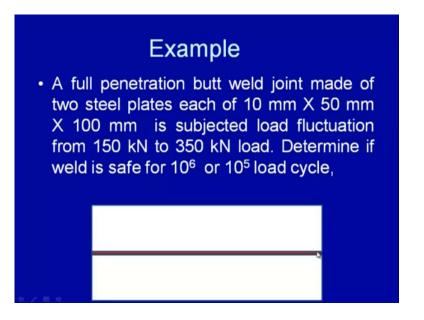
So, we will see one example to show that, the how the weld joint can be designed for the fatigue loading. Say for example, a full penetration butt weld joint made of the 2 steel plates, each of the 10 mm thickness 50 mm width and 100 mm length is subjected to the load fluctuation from 150 Kilo Newton to the 350 Kilo Newton. Then determine, if the weld is say for 310 to the power 6 or 10 to the power 10 to the power 5 load cycles. So,
