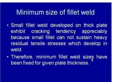
So, the minimum size of the fillet weld this is the reason, which has been explained the small fillet weld develop at, developed on the thick plate exhibit the cracking tendency appreciably. Because a small fillet cannot sustain the heavy residual stresses, which develop in the weld, and therefore minimum fillet weld sizes have been fixed for given plate thickness.
