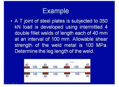
Now we will see one example, to show that how the design of the weld joints can be made. So, in the design of the weld joints, either we have to determine the throat thickness of the weld or the length of the weld. In such a way that the our weld load resisting cross sectional area can successfully, sustain the external load for a given allowable stresses.
