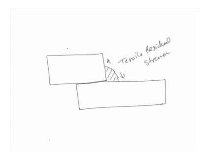
We can see that, if the plates to be welded are very thick and due to if we put in the fillet weld of very small in size, say of this. Then due to the development of the heavy tensile stresses, tensile residual stresses acting on the fillet weld will tend to crack it.
