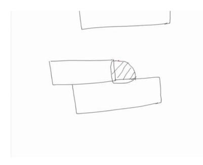
In case of the fillet weld minimum fillet weld sizes have been identified by and the American welding society and according to that some minimum size of the fillet weld must be deposited for the plate of the given thickness. And these dimensions minimum size of the fillet weld, which should be deposited according to as given by the American welding society will be shown in this in the next slide.
