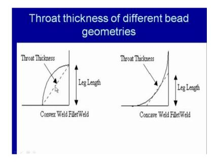
Using the various types of the geometries say for convex weld, the convex bead geometry is obtained in case of the concave fillet weld, this kind of geometry is obtained and to determine the throat thickness. One straight line will be which passing, through the fillet weld shortest length of a straight line passing, through the root of the fillet weld will give us the throat thickness.
