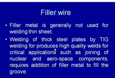
1 mm thick sheet is welded by directly melting the edges of the plates and allowing it to solidify to obtain the metallic continuity. But when thick sheets and thick plates are welded by GTAW process, the filler materials in form of rods invariably used. This is commonly used in case of the nuclear and aero space components. Under those conditions when thick plates are to be welded, the filler material is added in form of the rods of the different sizes.
