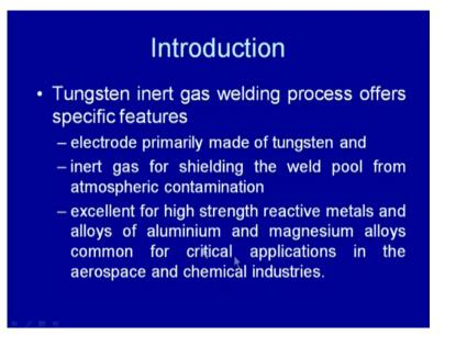
The weld joints as for and very clean weld is also produced. So, if you see the important features of this process, it basically use is the tungsten electrode, which is non consumable kind. It uses very inert gases like helium and argon to protect the weld pool. These in turn help in developing the sound and quality weld joint. Further, this effective shielding associated with the GTA process due to the smooth and stable arc and short arc length helps in developing the high quality weld joints.
