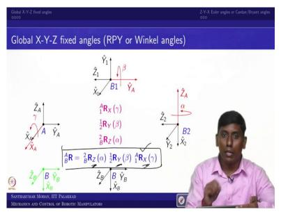
So, for understanding that we have taken two frames, so where A is the fixed frame and B is the final body frame, so now you can see that these two are having different representation. So at least we can see like three orientational information is required. Straight forward you cannot get simple with one or two rotation. So in that sense what we can try to do we will start rotating with respect to x axis.
