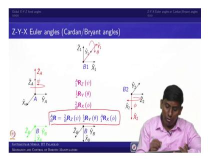
So let us go to the next one which is we call the same thing but we are writing in a moving frame which we call cardan or Bryant angle where we have taken this and we are trying to find. So in this case what first so first z axis rotation so then y axis rotation finally will come with x axis rotation. So, but what with respect to the moving frame? So in the sense right now we assume this is a moving frame so I rotate about this.
