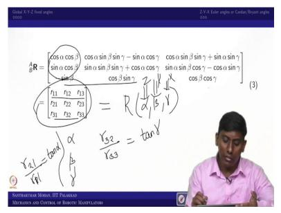
So this is the bigger matrix. So I have taken the same matrix but I have taken a conveniently safer place where you can see. So now this is equal into what I am writing as r 1 1 to r 3 3. So now what this? This is equal into R you can say alpha, beta; gamma where alpha is a rotation about Z axis. So beta is rotation about y axis this gamma is rotation about x axis. So I want to find out what is alpha what is beta and what is gamma if I know this value.
