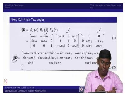
So this is the x axis rotation and this is the y axis rotation and this is the z axis rotation you multiply this end. So you will get this bigger matrix. So this bigger matrix is what so this is what the rotation matrix of B with respect to A. So, now if you are taking this into consideration, so what would be this equal into?
