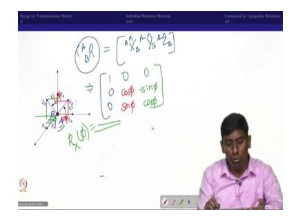
For going to that so, we will first of all talk about individual transformation, in the sense, individual rotation matrix. For example, I have a frame A. So, now, there is a body which is associated with the A in such a way that initially the X axis coincide here, I bring the B frame where the XB unit vector and the XA vector coincide.
