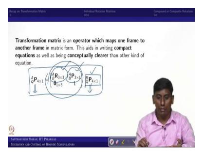
So, if that is the case, we can see like we will take the recap on transformation matrix. So, transformation matrix we know like it is an operator, which maps one frame to another frame in a compact matrix form. So, this aids writing a compact equation as well as the conceptually clear than the other kind of equation, in the sense, you can make one body to another body like that you can stack each box would be represented as a transformation matrix.
