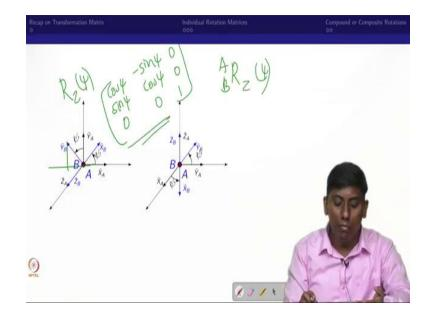
So, this is what we did here. So now the angle we call psi. So again, you can see like it is not so very clear. So we will take the same way. So, we will put ZA cap is coming out of the screen and we use the X and Y on the screen. So, now in that sense, if I rotate what happened, this would rotate and this also would rotate.
