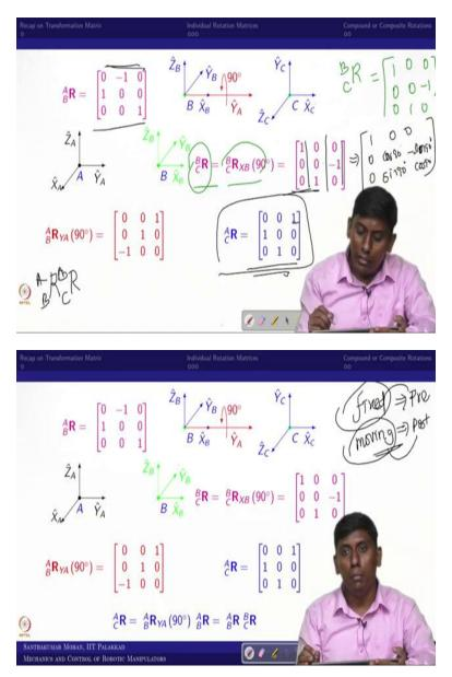
So, for that what we are taking it, we are taking it so the RB, so I am taking RCB, so that I can see. So, XC is projected on B frame where it is coincide with XB so 100 so where this YC is projected on ZB 001 and where this ZC is projected on Y, but opposite, so it is 0 minus 1 0. So, this is what we have written as RC with respect to B rotation matrix of C with respect to B.
