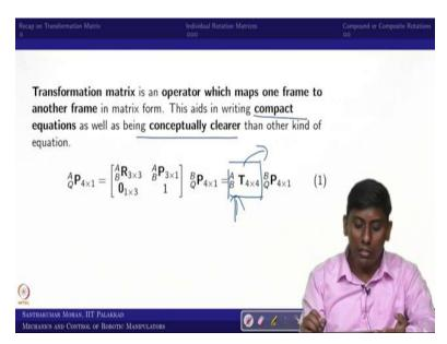
So, now, based on that what you can see the transformation matrix is four cross four, and this is what we are say saying that compact equation or compact form and it is conceptually clear, it would be having a homogeneous where the rotational and positional information is inbuilt.
