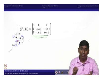
So, now, I hope this is what we have written so, the rotation matrix of B with respect to A where the rotation happened only with respect to X axis within a phi angle. So, then we can write the rotation matrix in this form, this is what we have seen.
