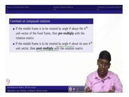
So, what comment is if the mobile frame is to be rotated by an angle theta, about kth unit vector of the fixed frame, then you pre multiply with the rotation matrix whereas if it is rotated by an angle about its own kth unit vector, then you post to multiply with the rotation matrix. I hope you are clear on that.
