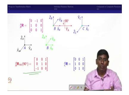
So, for understanding that more clarity or more clarity manner. So, I brought 2 frames. So, just to give a clarity, so, what clarity says that there is a frame A and B which are put it here. So, now if you look at it here, the rotation matrix of B with respect to A I can simply write like XB can be projected on A frame. So, in that case what happened this would come 010.
