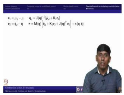
Welcome back to the you can say Mechanics and Control of Robotic Manipulator. Last class, we have seen like how the task space, you can see motion control can be done in MATLAB simulation. This particular lecture is in addition, so, again we are trying to do the MATLAB simulation but with what you call the cascaded or the double loop control scheme.
