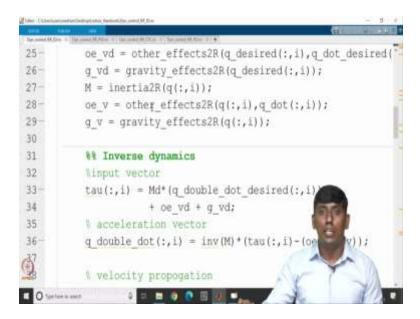
So, we will go to MATLAB code. So, you can see this is the code which we have shown there. So, you can see like this is inverse dynamics simulation of RR planar serial manipulator or robot. So, these are the cases so, now, we are taking it these all. So, here we assume that gravity is 0 later on we will bring it and here we are not considering the frictional effect because the frictional effect is not exactly model it.
