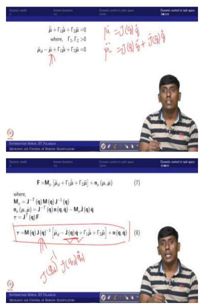
So, we used what we know; so again, we can come back to the second order error dynamics is going to be a stable system; where gamma1 and gamma2 are positive constants. So, only thing, so earlier we have taken q tilde double dot and q tilde dot and q tilde; so here mu tilde double dot. So, we can rewrite this equation, so we know mu double dot; so how we can write?
