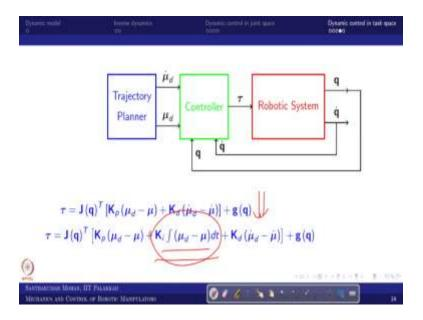
So, then we will go to the computed velocity control or computed torque control in this case. So, we will see this is the controller, the controller required feedback; and required input from the trajectory planner. So, then if it is a PD control, we can use it this way; but you need to give the input in task space. So, we know J is actually like, so the tau is J transpose of, so q into F.
