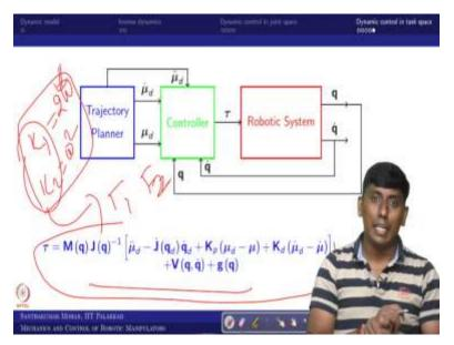
So, you can see this is the system and this is the controller; we take feedback, and we give three inputs from the trajectory planner. Both, earlier we give only desired position velocity; now desired acceleration also we added. So, then what happened this is the control law which comes to us; so, this is the computed torque control.
