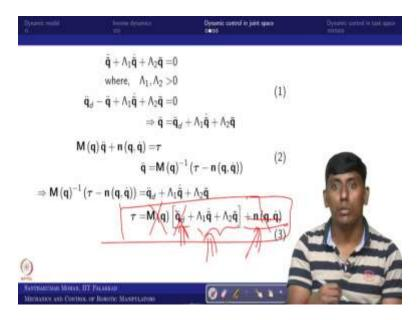
So, where lambda1 and lambda2 are a positive constant; in this case it is a matrix. So, we assume that it is a positive constant then we can see; so, this would be fulfilling what you wanted. So, we expand this equation, so we expand this q tilde double dot as q double dot desired minus q double dot. So, this q double dot we know from the equation of motion, and q double dot desired is available from the trajectory planner; so, this is what we can write it.
