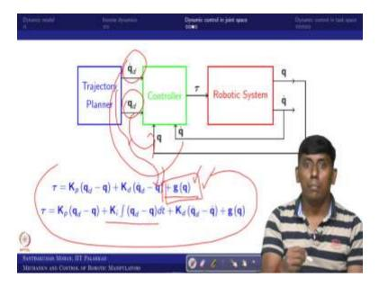
So, for that what we are taking it; so, before going to see that so we can see like the same thing in a block diagram form, so, this is the control. So, now we assume these two are fedback, so now that fedback and the trajectory planner is giving the q dot desired and q desired. So, then what we can see like this is the simple PD control along with gravity compensation. The same thing can be extended with PID, so then i term is coming again.
