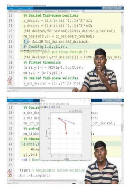
So, I will just write J, so which means so I just see this; so I will just take it. This is a J, which is from the q; so, this is; so, q of 1 comma i comma q of 2 comma i; in the sense theta1 and theta2. So, now I calculated J, so J I calculated; and then this is going to give. So, now instead of this J if I do it, so the nature will not be changing; so that is what I wanted to show it here.
