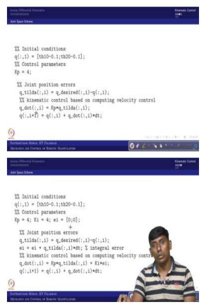
You are assuming that the q dot desired is unknown to us. So, then what happened the Kp we have taken; and Kp q tilde is the q dot. So, the q dot desired will not be coming into a picture; so, this would be having what we have seen in the last lecture. This would be having some steady state error; so that steady state error can be overcome with the integral control.
