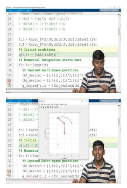
If I run this so what you can see this is the desired, and you can see like the actual is different; because it is an open loop control; it does not know how to correct it. So, in order to make it that clear for example, the initial conditions are same as the desired initial conditions. So, then you can see this would be giving the same trajectory following you can find it already; so, this is what we can see this particular plot is just for making more beneficial.
