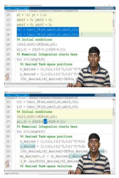
So, this is the inverse differential kinematics of the task space. You can see like this segment are same and the input whatever we have taken is same. So, only thing the trajectory coefficients we are calculating for x and y; so, because of that the x desired and y desired we are getting. Similarly, x desired dot and y desired dot we are getting. The same profile we have given and here also we have given induced this error.
