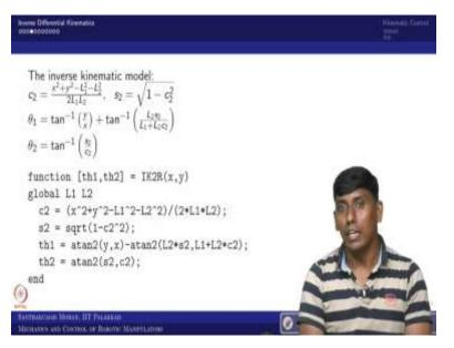
So, the same way we want to know like what is inverse kinematic model; because any of q desired, we would be taking from the mu desired. So, in that sense we need to know this; so, we are taking a inverse kinematic model which we have derived in one of the lecture, the same model we are taking it in MATLAB function. So, you can see this is going to return theta1 and theta2, for given x and y right. So, now these two functions are sufficient; so, then we need to know Jacobian.
