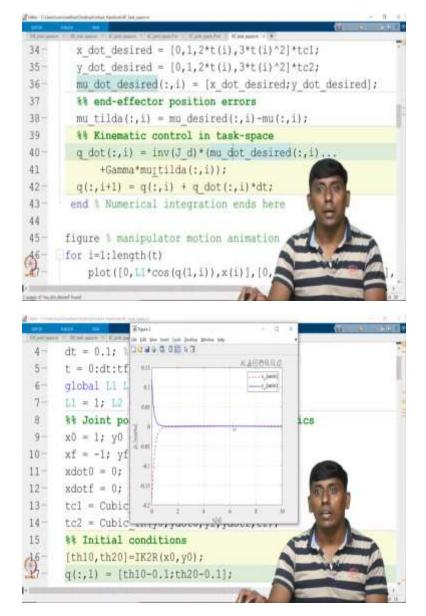
So, the mu tilde we calculate mu desired minus mu. So, then the q dot is inverse of Jd or inverse of J, multiply with mu dot desired plus gamma into mu tilde. So, now again we see that he initial is having error and this is a profile we want to follow, which is a straight line. We will see whether this is following it or not.
