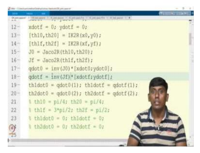
So, here I will just so correct this, so this is one thing which; because mu is like mu dot equal to J of q into q dot. So, we are trying to find out q dot; so obviously inverse of this. So, now these are
