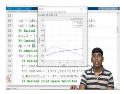
So, we have added Ki into ei; so, for that we have taken ei. Ei is ei of previous plus q tilde integrated; so, this is the integral error. So, now if I add Ki some value, so here we have taken as 4. If I added this what you can see the same condition; so, you can see like the error would be reduced. So, when t tends to infinity, it would be like see.
