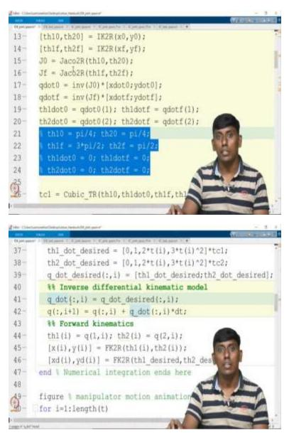
So, then we can use this, so instead of using the inverse differential kinematics and inverse kinematics; we can directly use this, so let us go to the initial condition. Now, we are taking as an open loop control, so theta1 desired and theta2 desired we have derived; and theta1 dot desired and theta2 dot desired also we have derived. And then we are using this inverse differential kinematic model what it says?
