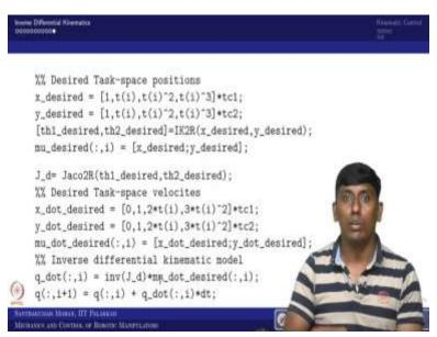
So, this is the task space, so now what change you can expect? So, the theta1 desired and theta2 desired become x desired and y desired. So, now theta1 desired and theta2 desired you want;
