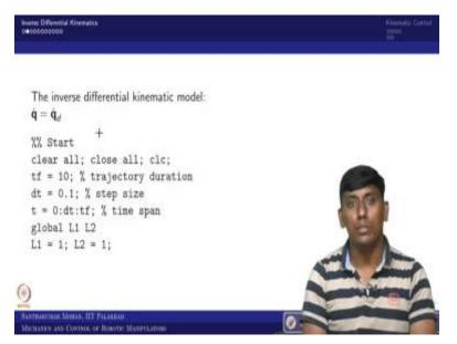
So, for that we are saying the first one is in the joint space, where q dot can be considered as q dot desired; this is the inverse differential kinematic model. So, here we assume that it is straight forward, so where the desired is known and we are assuming that is the actual; so, then we can write the MATLAB code in this way.
