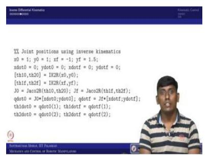
So, in that case, so we assume that the initial position and final position of the end effector is given, and the time also given already tf; so, which is 10 second. So, now we assume that it is a 2R serial manipulator, where L1 and L2 also given.
