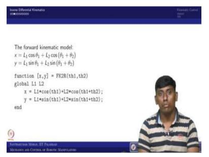
So, what we are trying to do the forward kinematic model, we want to use it; so x and y we want to write it, so, the x and y write it in this form. So, the same thing I can write as a one of the sub functions, where function x comma y basically this particular function would be returning x and y, for given theta1 and theta2.
