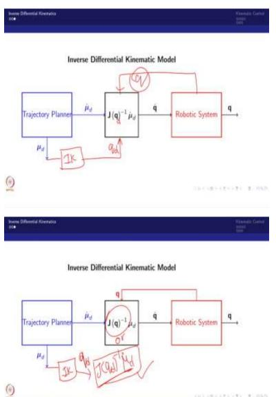
So, here we will see in a block diagram based. So, the robotic system will give as per kinematic level. So, it would be given as q output; and what would be the input, so q dot; so this is what we assume. And the inverse differential kinematics means what happened? So, there would be a trajectory planner. This trajectory planner will give what?
