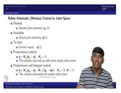
We can see how we can expose to simple feedback with a without even feed forward. So, for that we assume the initial thing all are like same; only thing the q desired dot is like is not available to us. So, then what one can do? We can simply calculate the error; and we can make it a simple proportional constant.
