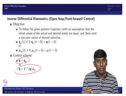
So, that conditions I am trying to put it here. So, what conditions? So, the objective here to follow the given position trajectory; however, what assumption explicitly given, so, with an assumption that the initial values of the actual and the desired states are equal. So, q of 0 and q desired of 0 are same; that is what we are written it.
