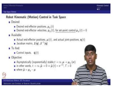
For the task space, what would be given? So, instead of desired joint position; it would be given desired end effector position; desired end effector velocity. And if it is a set-point, the desired end effector velocity would be 0. Then what we are expected? It would be available, so the actual end effector position and so actual joint position.
