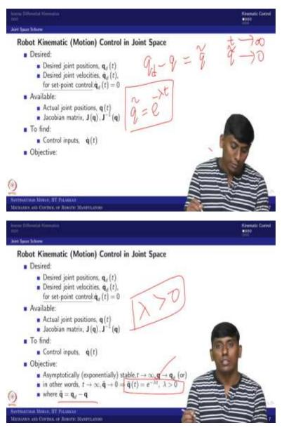
So, now we will move to the kinematic level control, where the joint space is the consideration. So, then the desired would be joint position, and joint velocity which nothing but q desired and q desired dot. So, if it is a set-point control, the q desired dot would become 0. So, then what one can thought about it? So, we can see what are the things supposed to be available?
