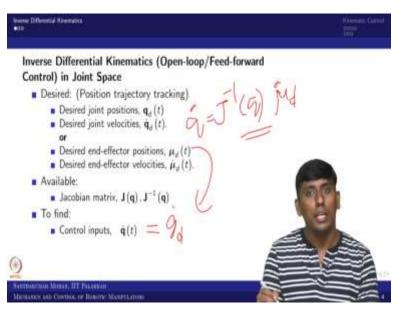
So, what inverse differential kinematics which we can consider as a feed-forward control; or we can say it is an open loop control. So, where we are end up? We end up with a joint space. So, in that case so what we are trying to see. So, the position trajectory is given; so, we have to follow that position trajectory tracking. So, what additional constraints would be given?
