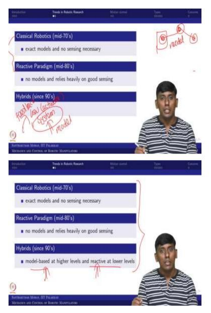
So, in that sense the exact models or no feedback are necessary. The exact model is necessary, and no sensing is necessary for this particular system. So, exact model is required, and no sensing is necessary for this system. So, it was working good as long the system is no wear and tear, or probably no compliance and all.
