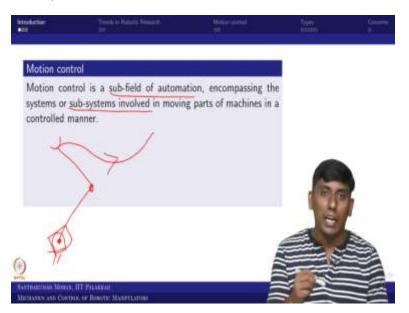
So, in that case first of all what is motion control? Motion control is a sub-field of automation. But what it is doing? It is encompassing the systems or sub-systems involved in moving parts of machines in a controlled manner. So, for example, I assume that this is the manipulator, which is having for example 2R serial manipulator which is fixed.
