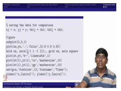
And the plot the individual animation we can try to show finally we will end with a comparative plot where you can say both trajectories how it looked like one is joint space, the other one is task space. How it looked like that we are trying to compare.
