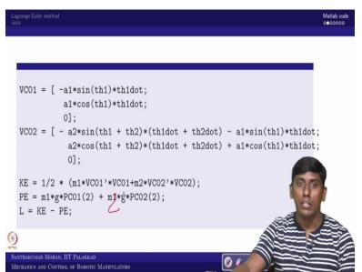
So, that velocity value I am rewriting in theta 1 dot and theta 2 dot manner. So, now what I got VC01 and VC02 and now what I wanted? I wanted the kinetic energy. So, the kinetic energy is half into m VC1 transpose VC1, VC01. So, this is what we have seen how to write in as you can see syntax and the similar way the second link kinetic energy also. So, here fortunate, there is no rotational kinetic energy, so we can leave it, only the translational kinetic energy we have taken.
