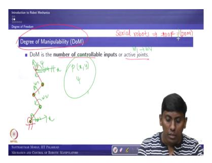
So, let us move further, we said one additional parameter you should know, what is that called degree of manipulability. So, what is manipulability? So, it is basically nothing but number of controllable inputs or active joints. By the name itself you can see if it is a serial Robot, if it is a serial manipulator or serial Robot, simply the serial Robot would be so the degree of freedom and degree of freedom and degree of mobility are same.
