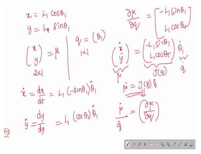
So, for example, x is L1, so cos theta 1. So, y is L1 sine theta 1, in the sense it is simple pendulum kind of thing, where L1 is constant. So, what would be this, so I can write x and y as mu. So, in the sense this is 2 cross 1. So, where q is only theta 1 which is 1 cross 1, what I wanted, I wanted I, so doh mu by doh q in the sense I can write this.
