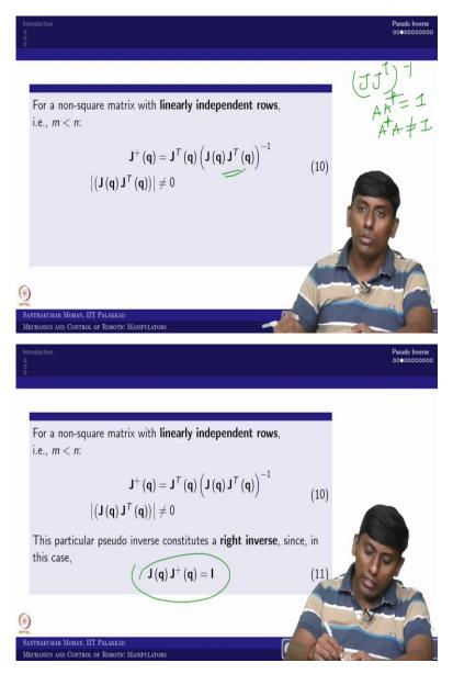
So, the other way around is like, if is m less than n in the sense, so it is for example, 6 is the mu vector, but you are n is more than 7 axes. For example, it is 7 axes in the sense q is like n cross 1 that is 7 axes in the sense this is having a 6 equation, but the seven unknowns in the sense it is under specified you have multiple solutions possible.
