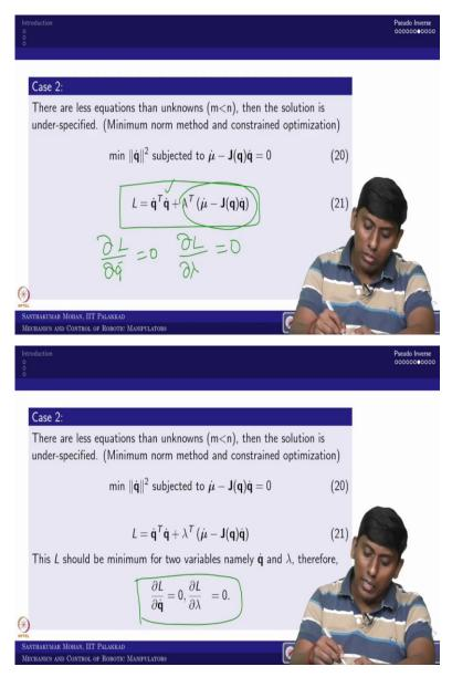
So, the next case is underspecified where m is less than n. In this case this is 6 and this is 7. So, in this sense it is actually like underspecified you can use a minimum norm method with the constraint optimization. So, what that means, so the q dot would be exists but multiple solution, so you minimize the q dot. So, in this sense you take 2 norm provided the mu dot minus J of q into q dot equal to 0, this is your constraint and you are trying to minimize this.
