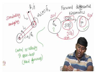
You connect you can say is, in the sense you take a serial manipulator. So, you take a motor, and you fix the rotational speed omega 1 and omega 2. So, in the sense or theta 1 dot or theta 2 dot. So, you fix it and L1 and L2 are known. So, you are trying to find out what is the x dot and y dot. So, in that sense what this is, this is straight forward. So, which we call forward, so differential kinematics. So, this is what forward differential kinematics.
