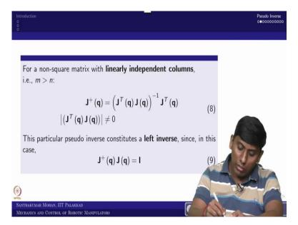
But if m is greater than n. In the sense, so, you have only 4 axes, but you have actual like spatial in the sense 6 DoF system, but 4 axes in the sense the q is having only 4, but the mu is having 6 cross 1. So, if that is the case what you have, you have 6 equations, but 4 unknowns, it is actually over specified, then what you can do you can do the left inverse. So, this is the left inverse where we have a square matrix J transpose J or J into J transpose.
