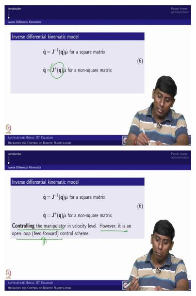
Whereas the inverse differential kinematics you can easily recall the J q inverse. So, in the sense it is like if it is a square matrix, if it is a non-square matrix, you would be using a pseudo inverse, which we have written as J plus. So, what this is equivalent, this is equivalent to controlling the manipulator in velocity level, however it is in an open loop control scheme in the sense it is a feed forward control, you please recall that, so it is a feed forward open loop.
