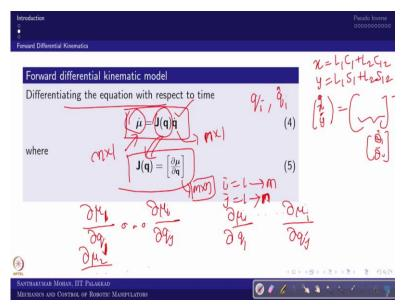
So, the same thing what we are writing in the other form. So, differentiating with respect to you can say time, differentiating the equation with respect to time, you can see that mu dot we have obtained as J of q into q dot, where this J of q is matrix of you can say partial derivative, why it is called matrix.
