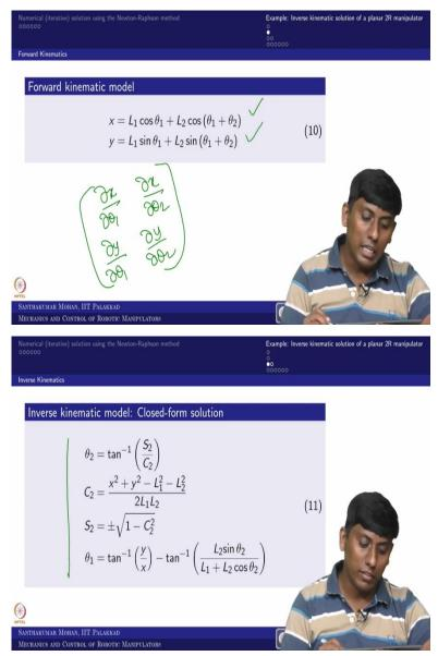
So, for that what one can do? We can go the Forward Kinematic model. So, this is what I have written. So, now you can take the partial derivative, what that means. So, doe x by doe theta 1. So, doe x by doe theta 2 and doe y by doe theta 1 and doe y by doe theta 2. So, this is what you call the Jacobian matrix.
