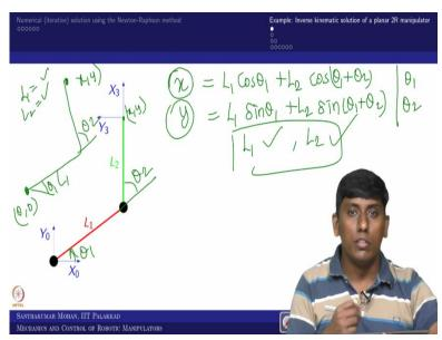
So now let us move the numerical example, for that we are taking a 2R serial manipulator. So, we know like this. So, what would be the x position of this, this is x and y. So, this x would be L 1 cos theta 1 plus L 2 cos theta 1 plus theta 2. So, theta 1 is this angle and theta 2 is this angle, so we can get this.
