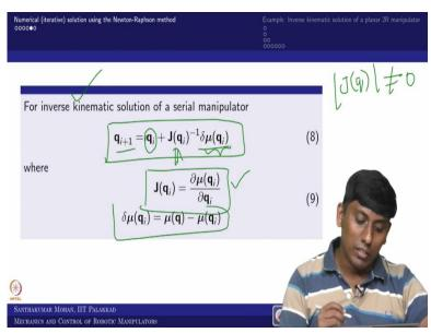
So, that is what we are trying to write. So now you can see that the, if the forward kinematics solution is available. We can find the inverse kinematic in iterative manner, where q i is the initial guess and J of q i is actually like based on the initial guess, what is the Jacobian matrix and this is actual minus, your function of q.
