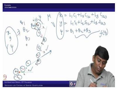
So, for benefit, I have just drawn that with some angle, you can see, this is the; you can say Z0 and Z1, where this is the frame 0 and 1. This is the frame 2, frame 3 and frame 4, where you can see each X axis aligned with the link and along this length, you got link length, L1, L2 and L3. And the angle between X0 and X1 about Z1 as theta 1, then angle between X1 and X2 as theta 2, X3 and X2 as theta 3.
