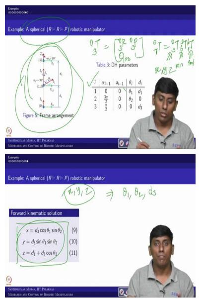
So, now I will just give only one slide further which is self-explanatory. So, you can see that the spherical robot, we have already, you can say draw the frame arrangement and we have found the DH parameter, and what we got, so we got finally based on the final transformation matrix of 4 with respect to 0. So, in this case, the T3 with respect to 0 will give rotational information of 3 with respect to 0, so these all we have seen.
