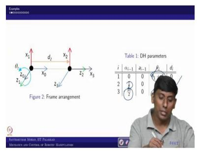
So, now this is the DH parameter, which is we obtained, so you can see which we have obtained. So, now what you can see, whatever we have written that all coming into a picture. So, this is the variable, and this is the variable. We can substitute this into individual arm matrixes and then we can see what is, you can call the DH representation giving finally forward kinematics. (Refer Slide Time: 10:38)
