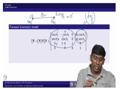
So, that we can substitute and finally multiply, you can see, this is the final multiplied matrix, what you get, so you can see that this is the position vector, which we have written, and this is the, you call the orientation or the rotation matrix. So, in the freezing point, theta 1 is actually like 0 degree. So, if you put 0 degree, what it is giving, so it is giving d2, 0, 0, that is what X displacement only there. So, you can recall.
