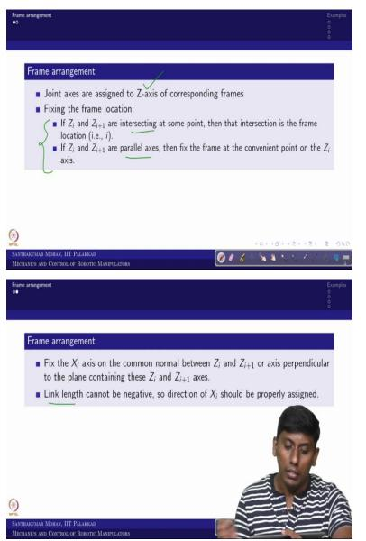
So, in that sense you can recall all those these things. So, we know like Z axis always associated with joint and the fixing the frame also like, if it is intersecting the intersection point would be the ith frame and if it is a parallel you can take convenient. Similarly, you can see like the X axis always taking a common normal, if the common normal is not there then the axis perpendicular to the plane containing the Z axis. And you can please remember that the link length cannot be negative.
