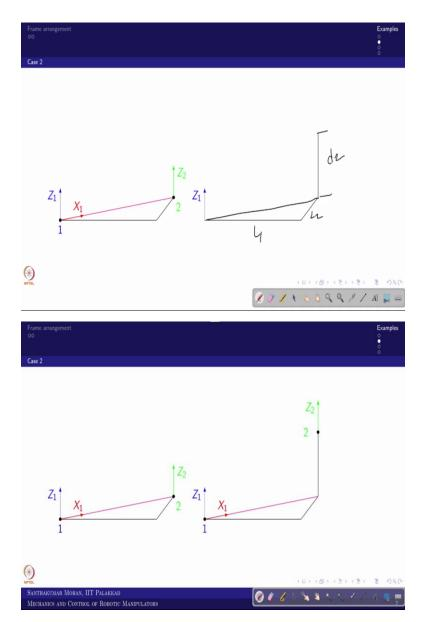
Which is little complex, what complex. I have taken the same plane, in the sense earlier also it is parallel, but now the parallel which is having off set it in both X and Y. So, in the sense you can see like this is in offset in 2 axis. How can we attempt? So, now it is you can draw a common normal, then there is a multiple common normal. So, what would be the best common normal, you will draw connecting this.
