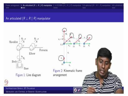
You can see, so this is what 0 and this is 1 and 2, and this 3 and 4, and we have fixed Z1, Z2, Z3 which are given and the Z0 and Z4 are choice. So, I keep it as per my want. And X0 to X4 we have to fix it. So, we have fix it based on the rule which we have used. So now, based on this what we have found, so we have found what you call the DH parameter. So, the same DH parameter what we have 10, we can cross check here.
