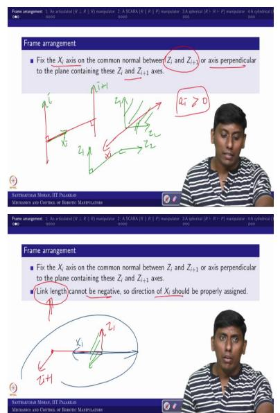
So obviously, then we have to see how to fix X. So Xi fixing is, always easy, because it is based on the nature of Zi and Zi plus 1. If it is parallel or you can say neither parallel, non intersecting, you can always draw the common normal between these two. And then you can fix along that as your axis. So, then that to like in the progressing side then that would be your Xi. This I say ith axis and this is i plus 1 axis you can take it.
