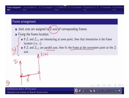
Let us go to the what you call frame arrangement, why we are thinking about frame arrangement, for example, you have several body, so how you can fix your joint axes, and what way we can fix the joint axes, if we fix the joint axes, where you can fix your frame, and where you can fix x axis, all those things you need to follow.
