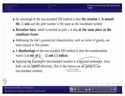
And the disadvantage always there. So, the disadvantage is mixed of the indices, what indices, so, i minus 1 and i would be inside arm matrix, where alpha i minus 1 and ai minus 1 would be exists, theta i and di would be other set. So, this is the disadvantage, but it is not going to create much confusion once you are getting familiar.
