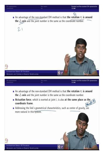
So, I will just end up with this to further slide. So, what is that, one is the advantage of having nonstandard is the rotation of theta i always around the Zi. So, in the sense you denote Zi as 1 and the theta 1 is corresponding to that, in the sense your actuator would be belongs to that, the joint number and the coordinate number coincide.
