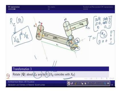
You can see that I mark it, so, Xi parallel at a point Q, which I am denoting as XR. So, now XQ and XR are angle apart, how much angle, theta angle with respect to what, the ZR. So, now what we can do, so ZQ and ZR parallel although, but XQ and XR are non parallel. So, you make it parallel.
