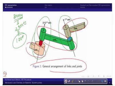
So, you can see right now, this is the general arrangement, we are trying to take the link i minus 1 which is connected link i and link i minus 2. So, obviously, you know like as per the Denavit-Hartenberg representation, what it says? So, any link is a binary link and each binary link would be, the name itself binary link. So, it would be having two joints and as per our case or as per the Denavit-Hartenberg approach. So, each joint would be having 1 DoF system or 1 DoF joints.
