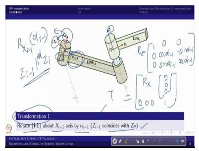
So, what else we can do? We can make it a parallel because we are interested to i, so we can a draw the parallel line to Z i with respect to the frame i minus 1. So, this is the parallel line. So, now what we are taking it, so we are from here, we are taking it one we make it parallel. So in order to make it Z i minus 1 and Z i parallel, so how much angle you have to rotate with respect to X i minus 1. So, that is what we already seen as alpha i minus 1. So, this is what we did.
