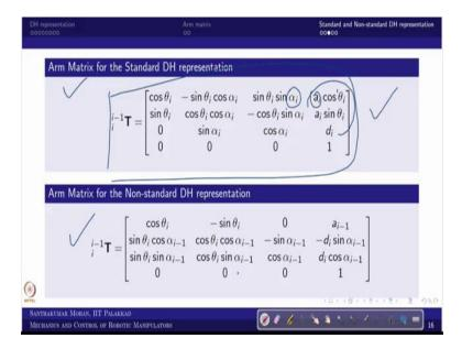
So, these are the two matrices will come. So, you can see very, very similar. So, this is the joint information is clear, but the link information is ai and alpha i is proceeding joint, the link parameter is relative information of 2 links, 2 joints so that would be in this case the proceeding link, but in this case, the current joint to the proceeding link and the joint angle also would be that way, the link to link and joint to joint which is exact correspondence.
