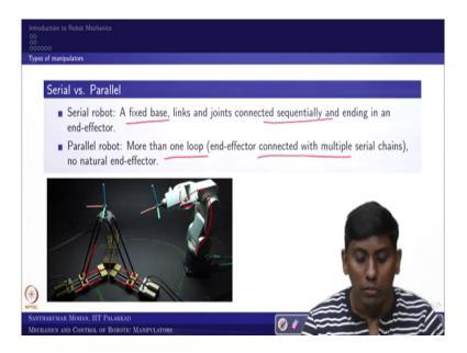
But, when we see the other way around the serial Robot we know though, one of thing is fixed based but the links and joints connected sequentially and the ending in an end effector. Whereas the parallel Robot more than one loop end effector connected with multiple serial chain. You can see, right. So, there are six actuators, but this is connected in parallel way. But this is open which is the serial chain.
