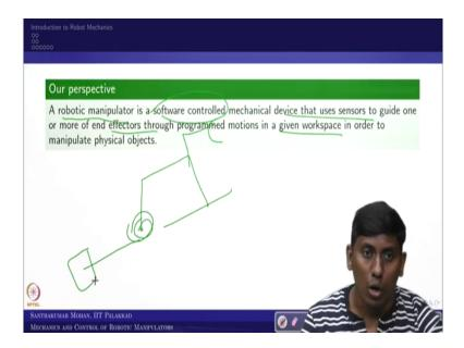
So, let us move further, so what would be our perspective of this course? So, we would be talking about robotic manipulator, that is nothing, but a software controlled mechanical device that uses sensors to guide one or more of end effectors to through programmed motion in given workspace to manipulate physical objects.
