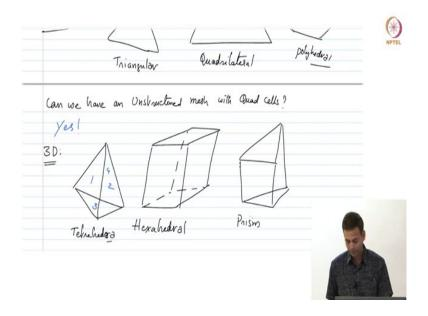
Now, can you have an unstructured mesh can you call an unstructured mesh with quadrilateral cells? Can we have an unstructured mesh with quad cells? We can have, right, ok. We can have. The answer is yes, ok. So, you can think about and come back to me later fine.
