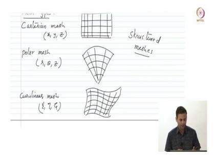
We can also have a mesh that is curvilinear, ok. Could also be some kind of a curvilinear mesh this could be in some generic coordinate system that is xi, eta, z, ok. So, this could, this may look like something like this. And these are all the cells that we may produce which are all curvilinear, depending on the shape of the domain we are trying to solve a particular equation.
