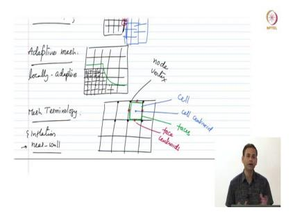
So, the terminology here is that, so the mesh terminology. So, as part of this course we will be looking at both structured as well as unstructured meshes and their treatment, ok. So, we will be solving some of these unstructured meshes. But they will be very simple. For example, I will give you an example as an assignment probably you will work with like 4 or 5 cells that are in an unstructured manner, ok.
