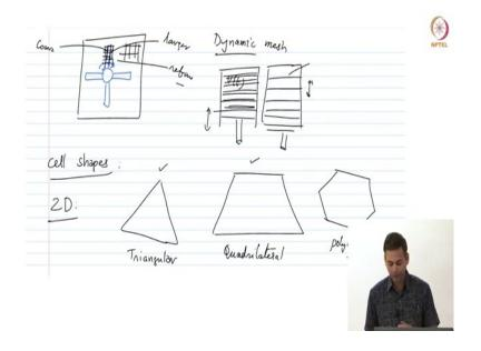
For example, take off this, for example, we can have maybe let us say a piston cylinder, ok, or maybe we want to solve for a wind turbine or something, so I have I have blades of this fan, which kind of rotate. Now, at particular instant I want to have the mesh to be very fine in these locations, right, but here I can have a larger mesh, right because this is where there could be large gradients, right.
