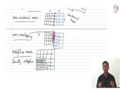
As of now I have drawn it as conformal, ok. So, these are now as I am sorry. As of now I would draw with a conformal mesh, ok. So, this is conformal. By conformal I mean that I have these two meshes and these nodes are matching at every location, ok, the kind of end at the same location we call it as let us say a conformal mesh.
