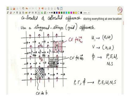
So, this is a very good remedy for avoiding checker boarding of pressure and velocity fields in the solution. So, we realized that we were actually getting checker boarding in the first place because of the way we have stored the velocities and pressures, right.
