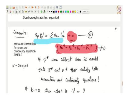
Now, what about Scarborough criteria for this? Scarborough criteria is it satisfied? Because we have to solve for a system here, is it not? This is an equation for a system of linear equation we have to solve for a pressure correction equation. So, we need to know
