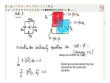
So, essentially the p if we if I plot only the cell p ok, this is what we have. Essentially we have P the pressure stored in the cell centroid and the horizontal x component of velocity that is  $u_e$  and  $u_w$  on the faces of the cell centroid, and on the north and south faces we have  $v_n$  and  $v_s$  stored ok, alright.
