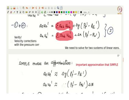
So, you need to verify how we got these equations. Basically subtract the equation set 1 from equation set 2, ok. Now, we got a very nice equation very important equation this is basically an equation that is relating the velocity corrections that we proposed with the pressure corrections, is not it? With the pressure corrections, with the pressure corrections ok. So, that is a very important equation.
