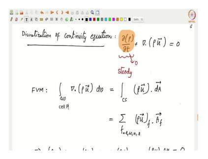
Then let us look at the discrete continuity equation. So, the continuity equation is basically  $\frac{\partial \rho}{\partial t} + \nabla \cdot (\rho \vec{u}) = 00$ , because we are assuming steady flow this particular term here is assumed to be this is basically goes to 0. So, we do not have  $\frac{\partial \rho}{\partial t}$ . So, only thing we have is  $\nabla \cdot (\rho \vec{u}) = 0$  ok.
