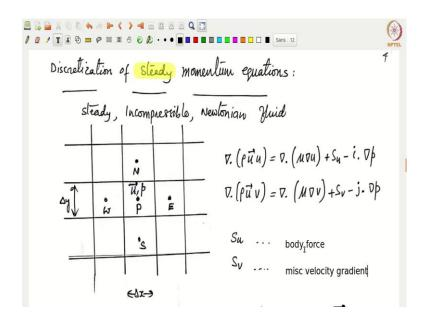
So, how do we now discretize the momentum equation? So, we would like to get kind of get started with a steady momentum equation ok. We do not want to do the unsteady as of now. So, let us make some approximations. The approximations we make are basically the flow is steady, and it is also incompressible, and the fluid we assume is basically a Newtonian fluid that means whose shear stresses are proportional to the strain rates ok.
