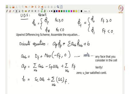
So, the upwind difference scheme we again recall from the structured mesh case that, phi all the face  $\phi_e$  is either  $\phi_P$  or  $\phi_E$  depending on the direction of the mass flow rate, right. If F e is greater than or equal to 0, then  $\phi_e$  equal to  $\phi_P$ ; if F e is less than 0, then  $\phi_e$  equals  $\phi_E$ , right we recall this thing.
