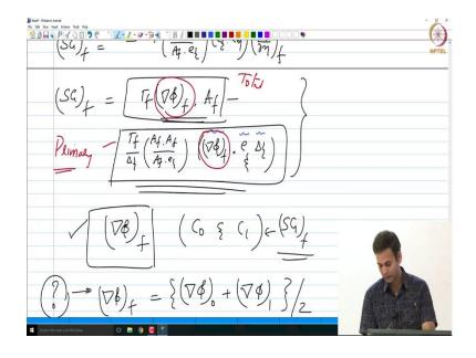
So, we have just transformed the problem of calculation of secondary gradient into calculation of gradient of phi on the particular face. Have you used any of these software the C F D software? It would ask you what is the gradient calculation scheme, right. Or some kind of how do you how should I calculate gradient? That is what it will ask you right.
