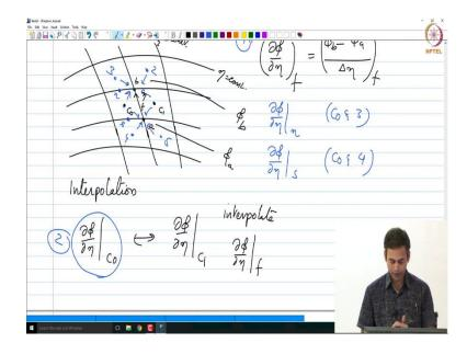
Instead of interpolating phi you can calculate what is  $\frac{\partial \Phi}{\partial \eta}$  at cell centroid  $C_0$ . And you can also calculate what is  $\frac{\partial \Phi}{\partial \eta}$  at cell centroid  $C_1$  and then interpolate these two to obtain what is  $\frac{\partial \Phi}{\partial \eta}$  on the particular face f that is shared between these two cell centroids right that can also be done right.
