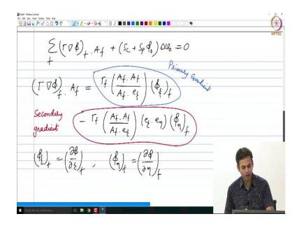
So, we said 0 cell is nothing but our p cell which is the primary focus and then we have three other neighbours which are one first cell second cell and third cell right. So, we have three more cells there fine then we formulated the value for the  $(\Gamma \nabla \varphi)_f \cdot A_f$  right.
