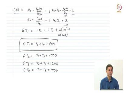
So, let us say a cell 1. What will be a east for cell 1 ok? Area vectors would again be same as delta y. So, we do not have to worry what will be a east?  $a_e = \frac{\Gamma_e \Delta y}{\delta x e} = 1$  for cell 1 right. What would this come out to be 1 ok, very good what about a north gamma north delta x by 1 y north what would this come out to be? 1 very nice. What about a west?  $a_w = \frac{\Gamma_w \Delta y}{\delta x b} = 2$
