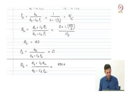
Then what is so, we are now at cell 2. So, what is  $P 2P_2 = \frac{b_2}{a_2 - c_2 P_1} = \frac{1}{2 - 1(\frac{1}{3})} = \frac{3}{5} P 2$  is b 2 by a 2 minus c 2 P 1. So, what is b 2? b is the coefficient of what? For cell 2 of T 3 right. So, that is 1 is not it, because b i T a plus 1. So, this is 1 upon, how much is a 2? a 2 is the coefficient of T 2.
