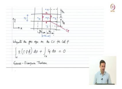
Now, what do we do, we invoke Gauss Divergence Theorem and going to convert this volume integral into a surface integral. So, this will be control surface gamma grad phi dot d A bar plus integral control volume S phi d v equals 0, that is what we have. Now what is this control surface in this context? Control surface is now made up of.
