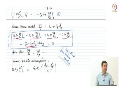
So, I am going to use a linear source model ok, which would tell me what is  $\vec{S}_{\phi} = S_c + S_p \phi_p$  So, we are going to use this source model, fine. So, if I were to put all of these back; what would that be?
