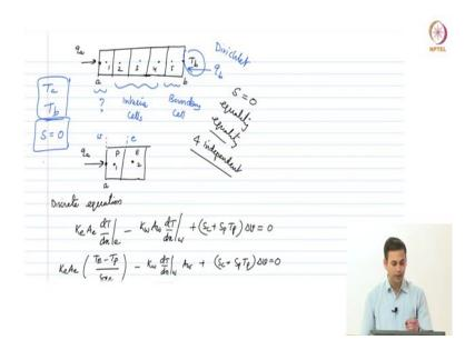
Let us get started. So, we were looking at the solving this 1 D problem which was basically we had a heat conduction problem right, where there are five cells with the given boundary conditions 1, 2, 3, 4, 5. And then we had a isothermal condition on the right hand side and there is a heat flux condition that is given on the left hand side; we called the faces a and b the end faces.
