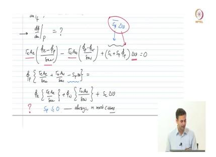
So, that would be you would have collect all the coefficients for phi P ok, phi P coefficients are what our gamma east A east by delta xe with a minus. So, we kind of send this to the right
