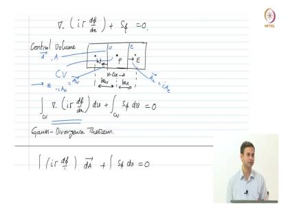
So, we have this kind of notation. Now, so the control volume we are focusing on is this guy this is the control volume, we will integrate our governing equation on this control volume as integral  $\int_{cv} \nabla \cdot \left( i\Gamma \frac{d\phi}{dx} \right) dv + \int_{cv} s_{\phi} dv = 0$ . Let us also assume that this is a 1D problem, let us also assume that the area of these faces of these east west faces is has a magnitude A ok.
