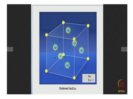
Now, we can do a similar exercise for the ordered Au Cu 3 and disordered Au Cu 3 you see in an ordered Au Cu 3 material the corner sides will be occupied by the gold atoms and the face centred positions are occupied by the copper atoms. So, the chemical you see one corner atom plus 3 of gold and 3 face centred atoms of copper. So, there are four atoms per unit cell in this particular case.
