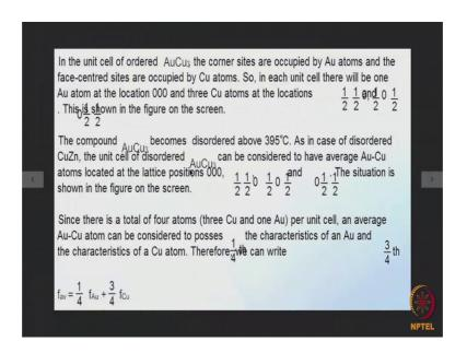
And again as we did with respect to Cu Zn we know that the in case of ordered Au Cu 3 in case of ordered Au Cu 3 we can find out that the corner locations are 0 0 0.
