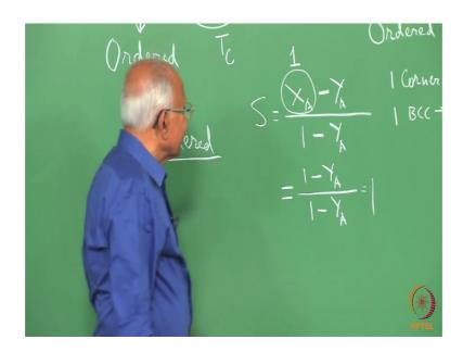
So, in case of ordered Au Cu 3 in case of ordered I am sorry ordered Cu Zn the degree of order is equal to X A minus Y A by 1 minus Y A where X is a fraction of a particular side which is actually occupied by the right kind of atom. So, here the fractions of corner sides are occupied by copper. So, entire this fraction all the corner sides occupied by copper in ordered condition, so, this fraction is equal to 1.
