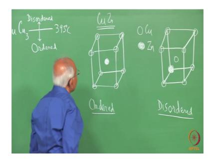
So, in Cu Zn in Cu Zn at low temperature when we say that it is in the ordered condition then the 8 corner locations are occupied by copper atoms and the body centred location is occupied by a gold atom. So, these are the copper atoms at the 8 corners of Cu Zn. So, these are the copper atoms whereas the one at the body centred position is a zinc atom.
