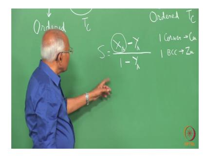
So, what is X A is a fraction of a sides which are actually occupied by the right kind of atoms now what are the 2 different sides available to the copper and zinc atoms in a unit cell of Cu Zn one corner side one corner site in the ordered condition by copper atoms and one body centred cubic side to be occupied by zinc atoms.
