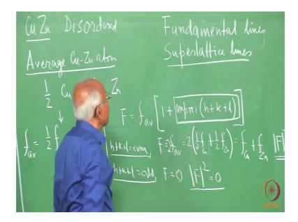
Those are known as the super lattice lines those are known as the super lattice lines; obviously, the intensity of the super lattice lines will be much less as compared to the fundamental lines because of this reason you know here f c u it is f c u plus f z n square in case of h plus k plus l is even and in this case when h plus k plus l is odd f square f c u minus f z n square naturally the super lattice lines are much weaker compared to the fundamental lines.
